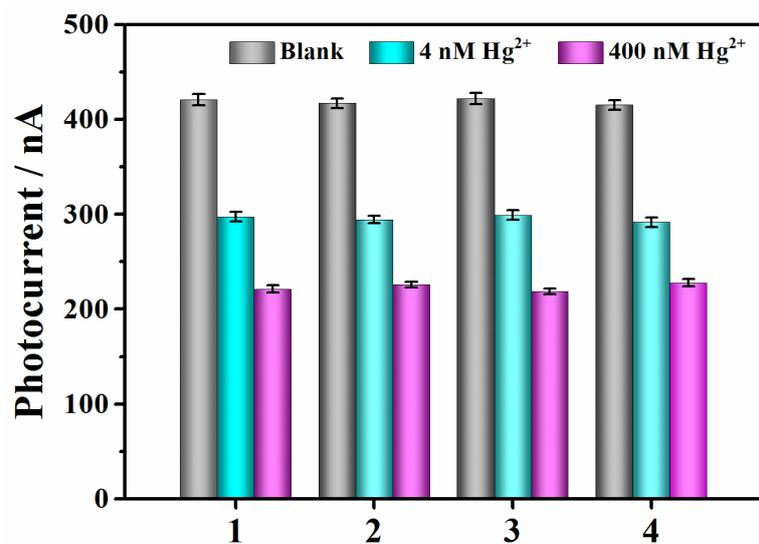
**Figure S2.** Photocurrents obtained on four different bare ITO electrodes in the absence and presence of 4 nM and 400 nM Hg<sup>2+</sup>. The other experimental conditions are the same as those mentioned in Experimental Section, and the error bars represent the standard deviation of five repetitive measurements.
