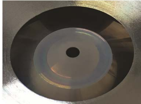
Figure S9: Lens contamination depending on matrix. Photo images showing the different lens contamination patterns after analysing 3072 spots with each matrix at the described laser powers in Table 2 and below.
