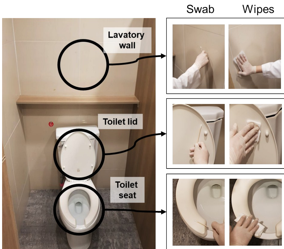
Fig.S4. Various surface measurements of lavatory for performance testing.
