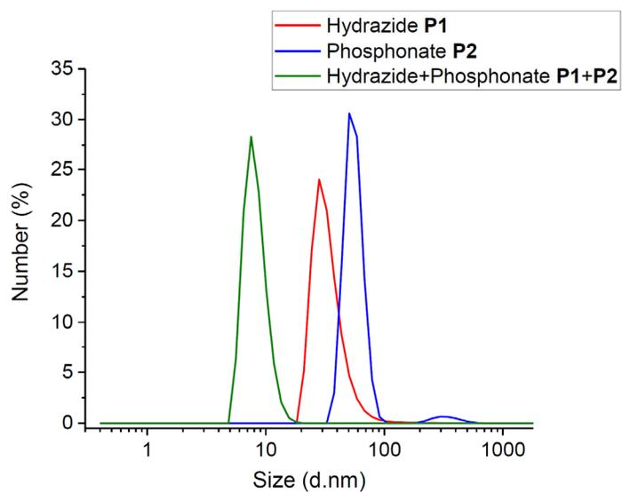
**Figure S2.** Dynamic light scattering data for nanoassemblies formed by polymers **P1**, **P2** and **P1+P2**.
