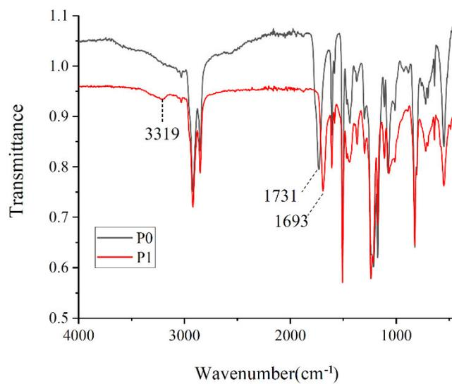
**Figure S1.** FT-IR of polymer carboxylate polymer **P0** and hydrazide polymer **P1**.
