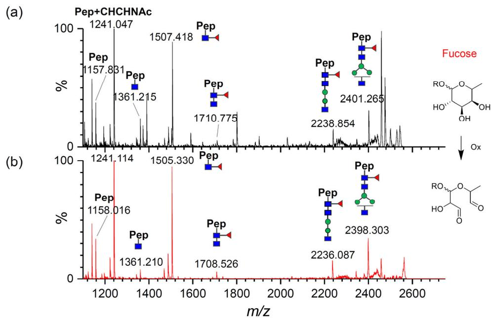
**Figure S3.** Glycopeptide analysis before and after enrichment with polymer **P1**. (a) Tandem mass spectrum of the precursor ion at  $m/z$  2602.1 from the IgG1 digest and (b) Tandem mass spectrum of  $m/z$  2600.4 after oxidation and enrichment (b). Symbol: (■) GlcNAc (●) Mannose (◄) Fucose.
