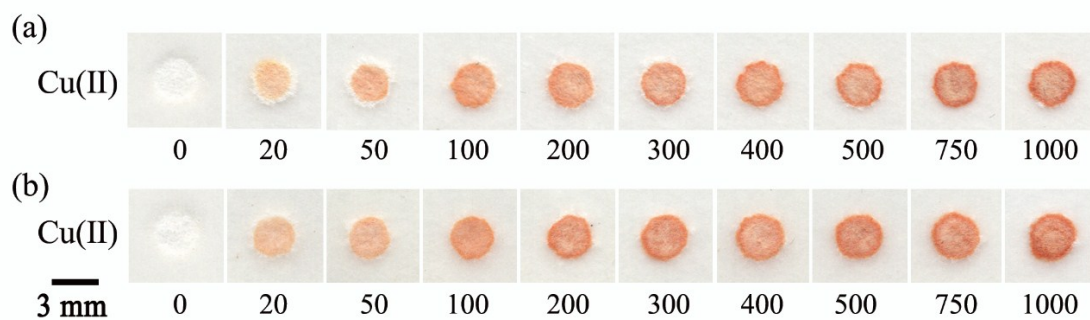
Fig. S5. The original optical images of the colorimetric assays for Cu(II) with different volumes of the sample: (a) 1.2 \mu\text{L} sample volume (b) 1.8 \mu\text{L} sample volume.
