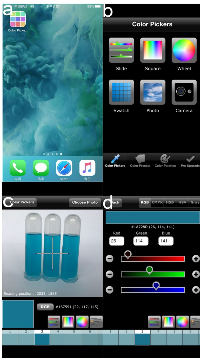
Fig. S7 Screen captures during the antioxidant detection by a smartphone: (a) iPhone menu loaded app, (b) main menu of the Color Pickers app, (c) typical sample analysis process, and (d) final results in RGB mode obtained after image processing.
