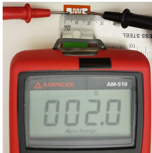
Figure S8: Low resistance microheaters are possible to create using the technique described in the main text. The design here has fewer serpentine turns resulting in a shorter path length. Specs: trace width: 0.529mm, path length: 24.264 mm, total heating area: 4 mm x 8.8 mm.
