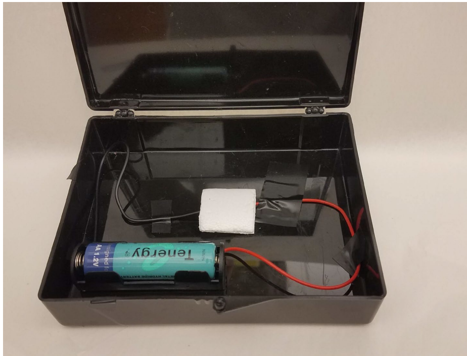
Figure S2: Setup for incubations powered by AA battery. Box was closed after initiation.
