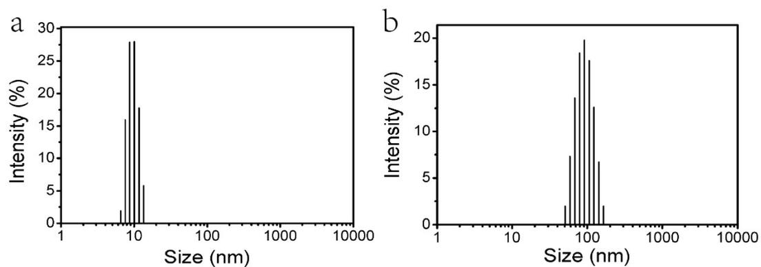
**Fig. S9** Size distribution of the probe solution determined using dynamic light scattering (DLS) method without (a) and with (b) incubation with NaHS (100  $\mu$ M) for 30 min.
