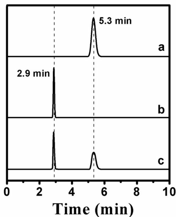
**Fig. S10** Typical HPLC chromatogram of Compound 3 (a), the probe (b), and the reaction solution after the reaction between the probe and NaHS for 15 min (c) from the 360 nm channel. And the mobile phase is methanol/H<sub>2</sub>O/acetonitrile (v/v 89/10/1).
