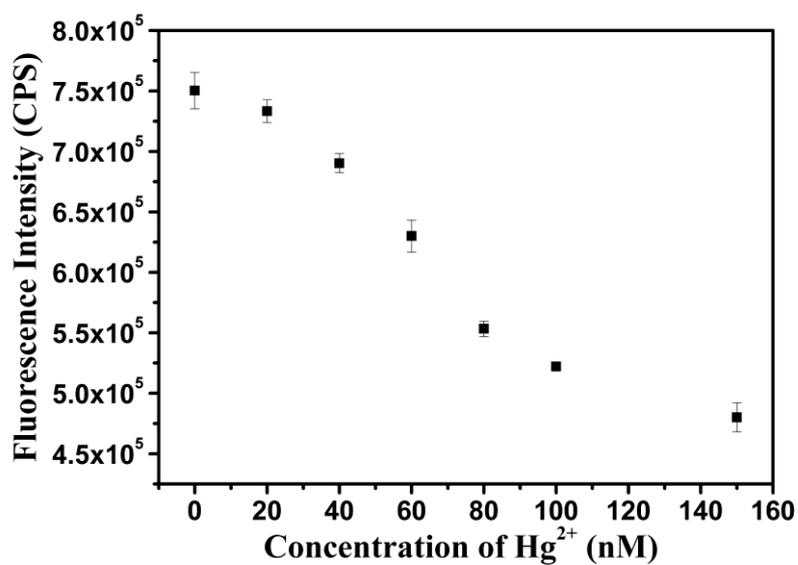
**Fig. S10** Scatter plot of fluorescence intensity of Baby Spinach-DFHBI complex as a function of the concentrations of  $\text{Hg}^{2+}$  (0-150 nM). The concentration of Baby Spinach is 100 nM, and DFHBI is 10  $\mu\text{M}$ .
