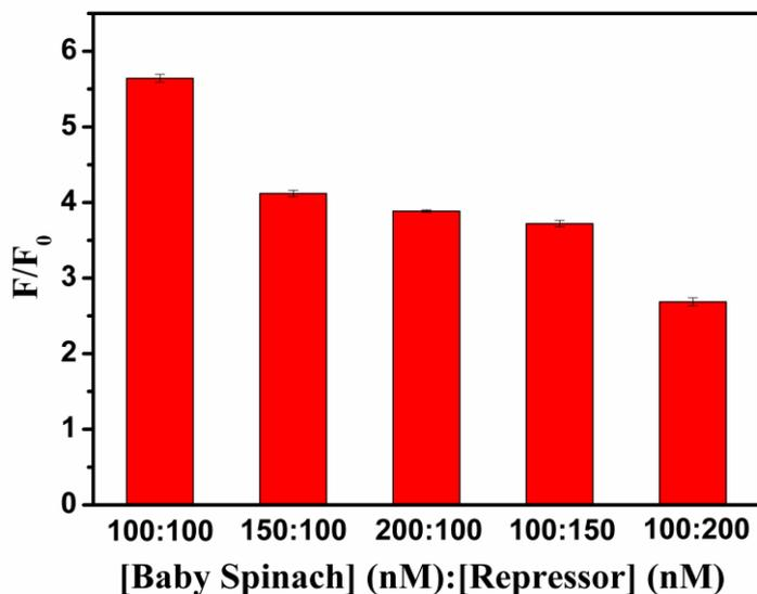
**Fig. S2** Optimization of the concentration of Baby Spinach and repressor strand for miRNA-21 detection. The concentration of miRNA-21 is 100 nM, DFHBI is 10  $\mu$ M. F and F<sub>0</sub> are the fluorescence intensity of the system with and without miRNA-21, respectively. According to the figure, 100 nM Baby Spinach and 100 nM repressor strand were chosen for further investigation to ensure the highest signal-to-background ratio.
