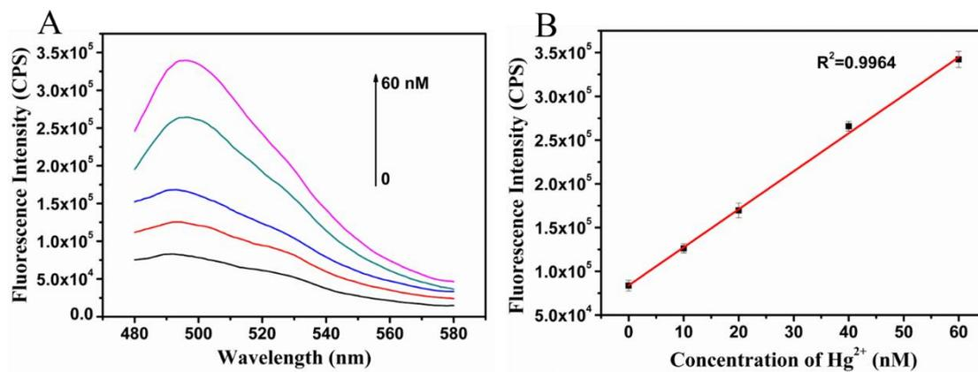
**Fig. S11**  $\text{Hg}^{2+}$  detection in seawater by using UBSP\_  $\text{Hg}^{2+}$ . (A) Fluorescence spectra of the system with different concentrations of  $\text{Hg}^{2+}$  (0-60 nM); (B) Scatter plot of fluorescence intensity as a function of the concentrations of  $\text{Hg}^{2+}$  (0-60 nM).
