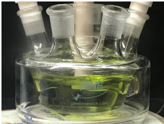
Figure S26 Picture of electrochemical cell containing 2 mM ferrocene in 0.25 M [\text{NBu}_4][\text{PF}_6] acetonitrile following final RDEV-OCP measurement. Solution color changed from orange – as expected for ferrocene – to green over the course of the scans.
