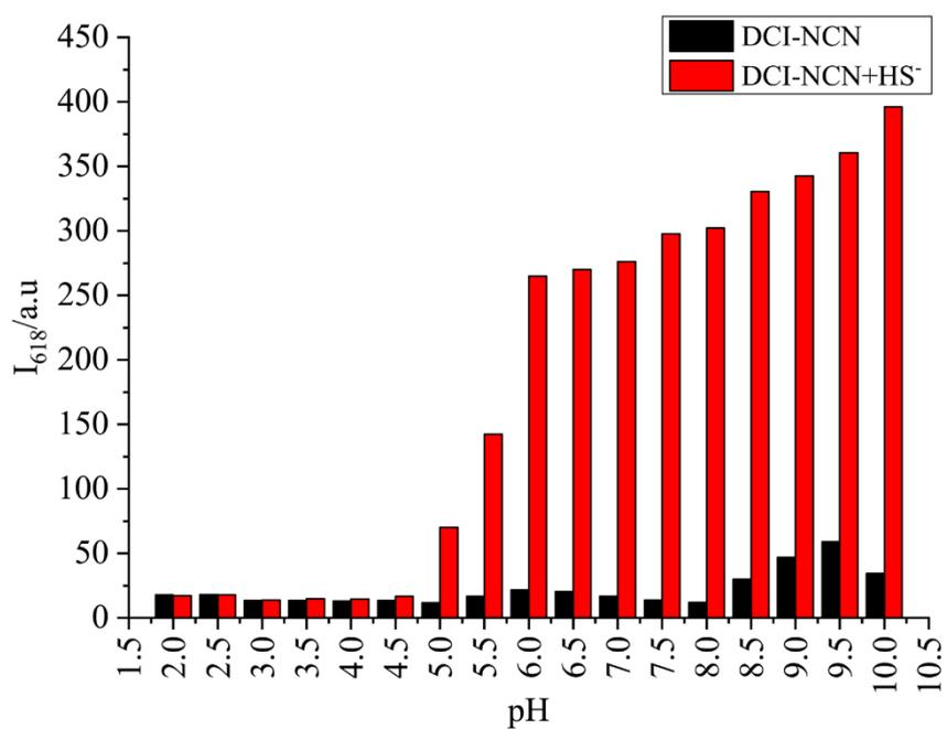
Fig. S3 Fluorescence intensity changed at 618 nm with Na<sub>2</sub>S upon different pH with  $\lambda_{ex}$  at 440 nm at 25°C.
