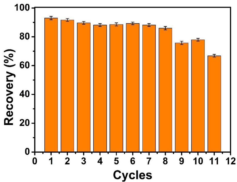
Fig. S5 The reusability of C-Co@PST sorbent for BPA extraction.
