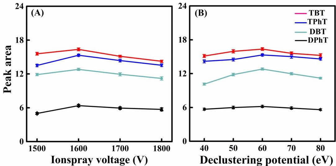
**Fig. S1.** Effect of ESI ionspray voltage (A) and declustering potential (B) on the sensitivity of four organotin compounds. Sample concentration: TBT (1 µg/mL), TPhT (10 µg/mL), DBT (10 µg/mL), and DPhT (10 µg/mL). The other instrument conditions are the same as shown in Fig. 2.
