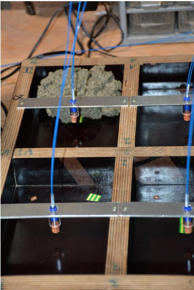
**Figure S4** Positioning of the four sensors during concreting.
