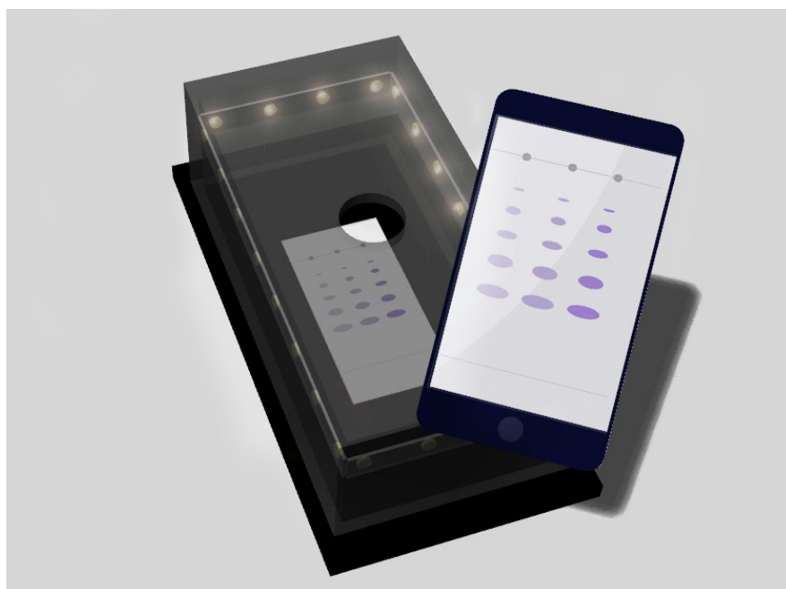
Supp. Figure 2. CAD drawing of the box used for homogeneous and reproducible lighting of TLC plates.
