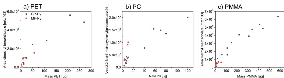
**Figure S3** Examples of calibration curves of CP-PyGCMS (black squares) and MF-PyGCMS (red dots) with higher polymer amounts outside the linearity range
