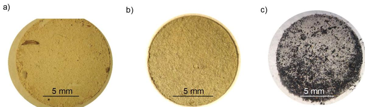
**Figure S4** Preconcentrated samples on glass fibre filters: a) salt sample, b) seawater sample, c) sediment sample.
