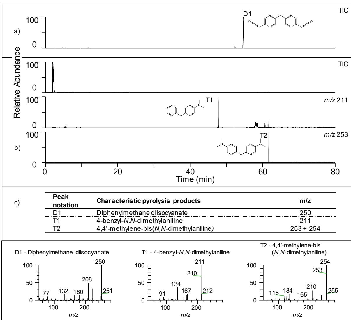
**Figure S2** MDI-PUR; a) pyrogram (TIC) of direct pyrolysis and b) pyrogram (TIC and selected ion chromatograms) of thermochemolysis of selected indicator compounds; c) table of characteristic pyrolysis products with d) mass spectra of these products.
