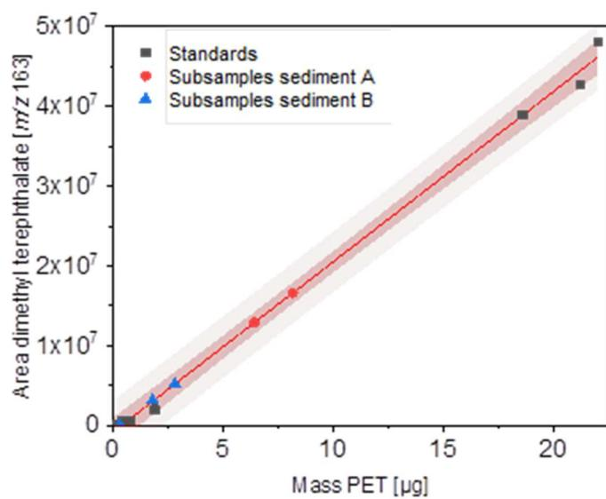
**Figure S5** Example of calibration curve (PET) for evaluation of sediments without addition of ISTD<sub>py</sub>, sediment sub-samples are visualized by red dots and blue triangles.
