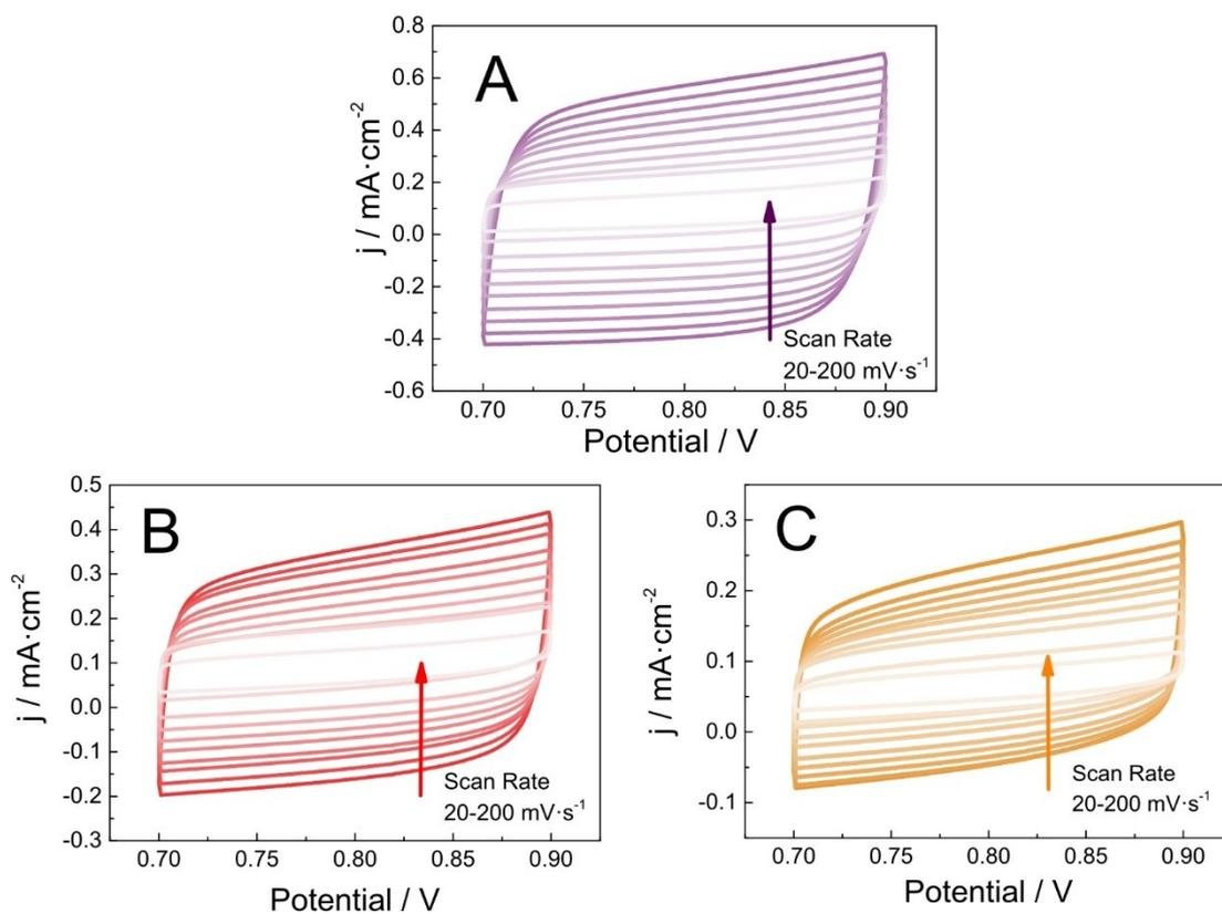
**Fig. S4.** Electrochemical surface area (ECSA) tests of MWNTs-COOH, o-MWNTs and raw MWNTs in 0.1 M PBS (pH= 5). Cyclic voltammetry curves of MWNTs-COOH (A), o-MWNTs (B) and raw MWNTs (C) with different scanning rates from 20 to 200  $\text{mV} \cdot \text{s}^{-1}$ .
