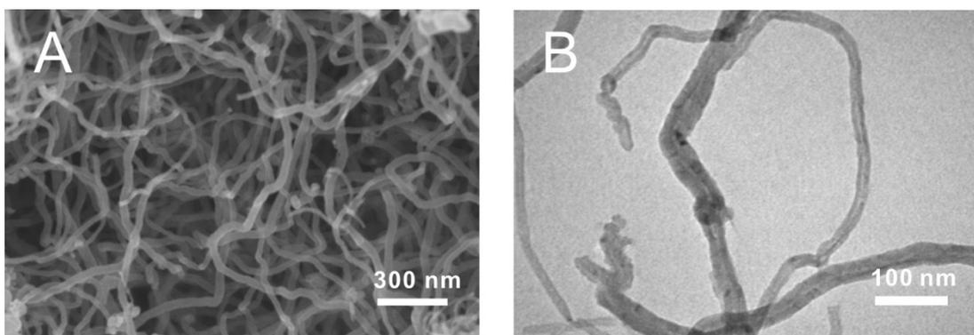
**Fig. S1** The SEM (A) and TEM (B) images of MWNTs-COOH.
