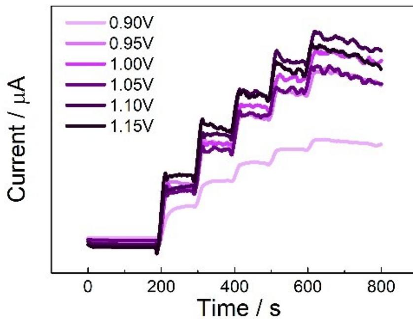
**Fig. S7.** Amperometric responses of MWNTs-COOH modified GCE for RhB at different potentials (0.90 to 1.15 V).
