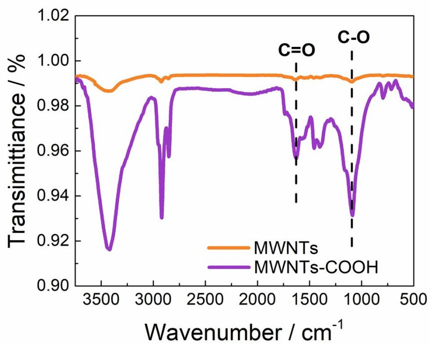
**Fig. S3.** FT-IR spectrums of MWNTs and MWNTs-COOH, and the image shows the characteristic absorption of C=O and C-O.
