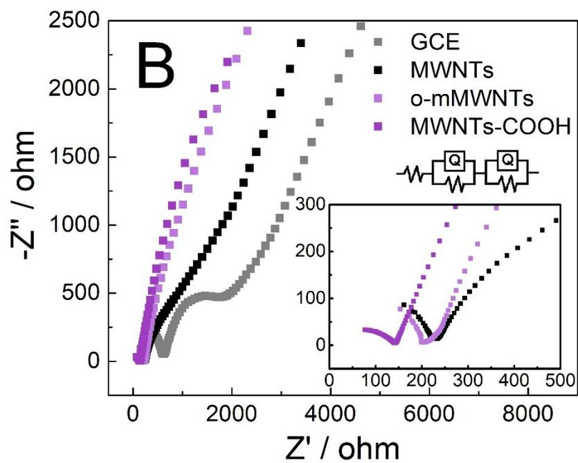
**Fig. S5.** EIS plots of bare GCE, MWNTs, o-MWNTs and MWNTs-COOH in 0.1 M KCl containing 1.0 mM  $[\text{Fe}(\text{CN})_6]^{4-/3-}$  with a frequency range from 0.1 to  $10^6$  Hz. The equivalent circuit was stimulated in the inset.
