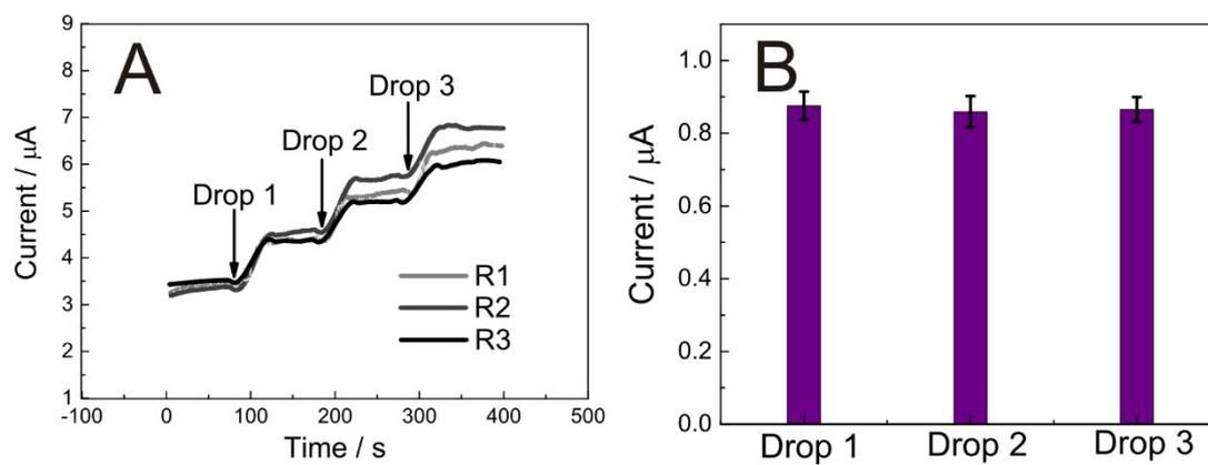
**Fig. S8.** (A) The reproducibility investigation of 3 amperometric experiments (R1–R3) with 3 successive dropwise addition of 5  $\mu\text{M}$  RhB; (B) The reproducibility investigation of 3 reduplicative experiments (Drop 1- Drop 3) for amperometric determination of RhB at the applied potential of 1.0V.
