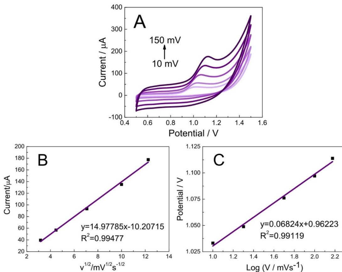
**Fig. S6.** (A) CVs of the MWNTs-COOH/GCE in 0.1 M PBS (pH=5) including 0.5mM RhB solution at different scan rates of 10, 20, 50, 100 and 150  $\text{mV s}^{-1}$ ; (B) The plots of peak current versus the square root of scan rate for RhB; (C) Plots of reduction peak potential vs.  $\log v$  for RhB.
