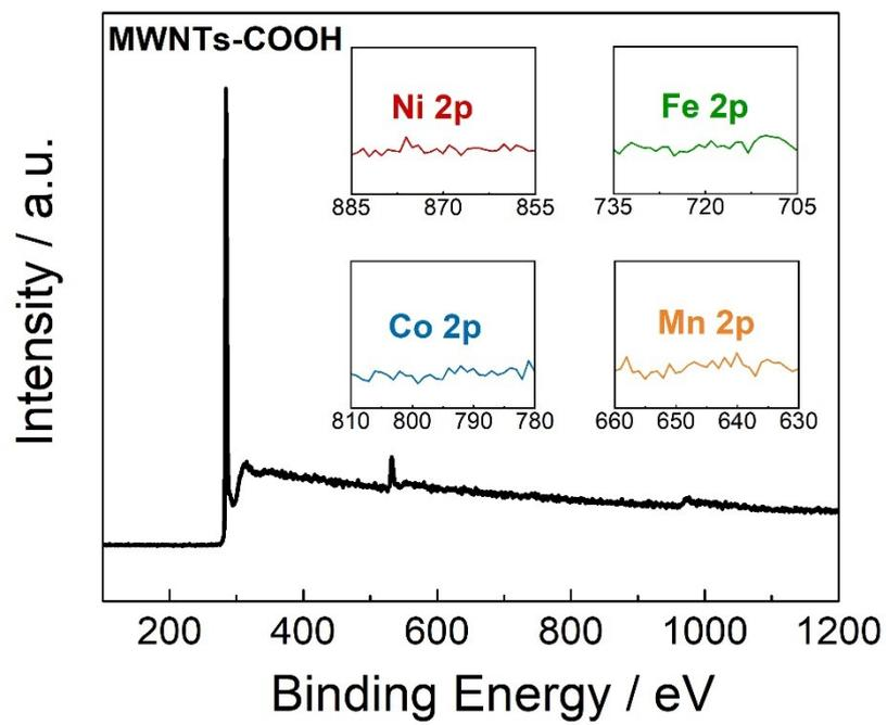
**Fig.S2.** The high resolution XPS survey spectrum of the MWNTs-COOH.
