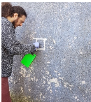
Delimitation of an approximate square of 100 cm 2 for the application of the Dust Wipe Method.
