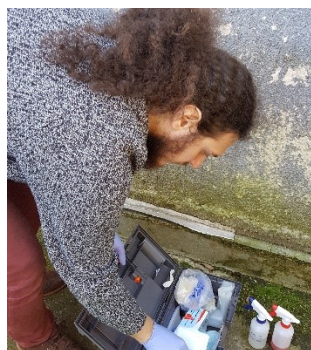
Carry-on kit containing all the elements for the application of the Dust Wipe Method.
