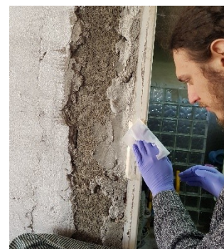
Scrapping a paint chip from an old recycled door employed in the construction of a new home.
