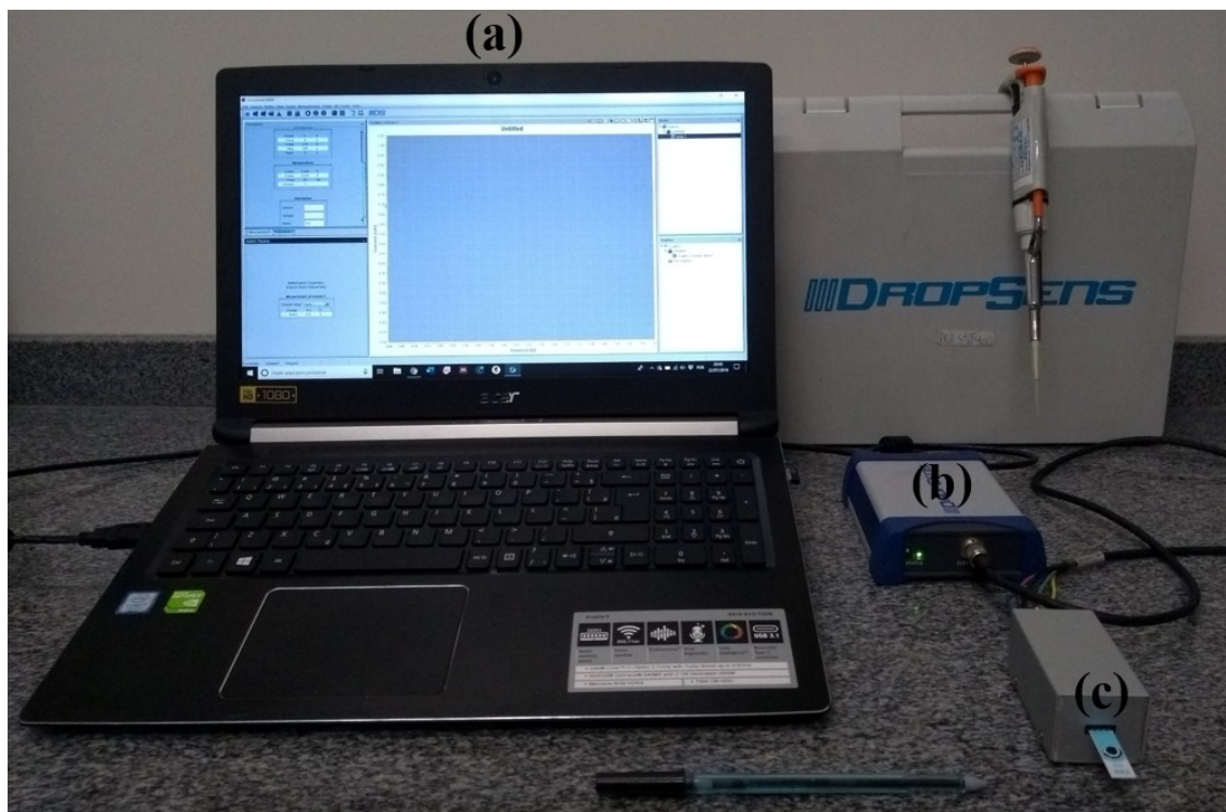
Figure S1. Electrochemical detection system: (A) notebook with software DropView®; (B) portable bipotentiostat/galvanostat model \mu Stat 400; (C) the screen-printed carbon electrode containing the sample.
