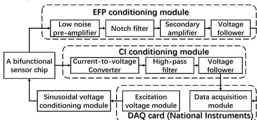
Fig.S1. The workflow of the platform hardware
