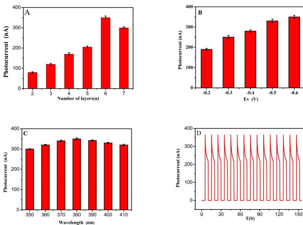
**Fig.S2** Photocurrent intensity of the CdTe QDs modified ITO electrode vs. the number of bilayers (n) of (PDDA/CdTe)<sub>n</sub> multilayers (A), applied potential (B) and (C) wavelength (D) time-based photocurrent response of the sensor. The photocurrent response was measured in 0.1 M PBS (pH 7.40) containing 0.1 M AA. The applied potential was -0.5 V. The light wavelength was 400 nm.
