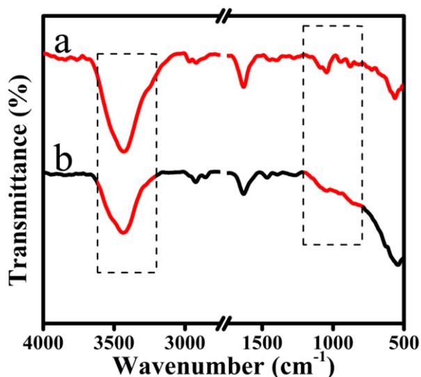
**Fig. S13** FT-IR spectra of N/S CDs with the absence (a) and presence of Cd<sup>2+</sup> (b).
