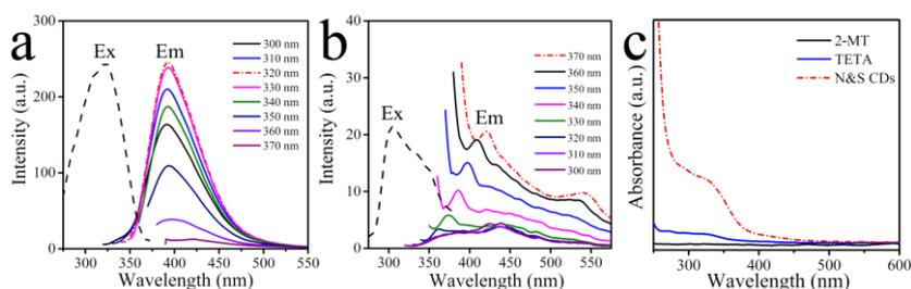
**Fig. S5** Fluorescence spectra of TETA (a) and 2-MT (b) UV-vis absorption spectrogram of TETA, 2-MT and the CDs (c).
