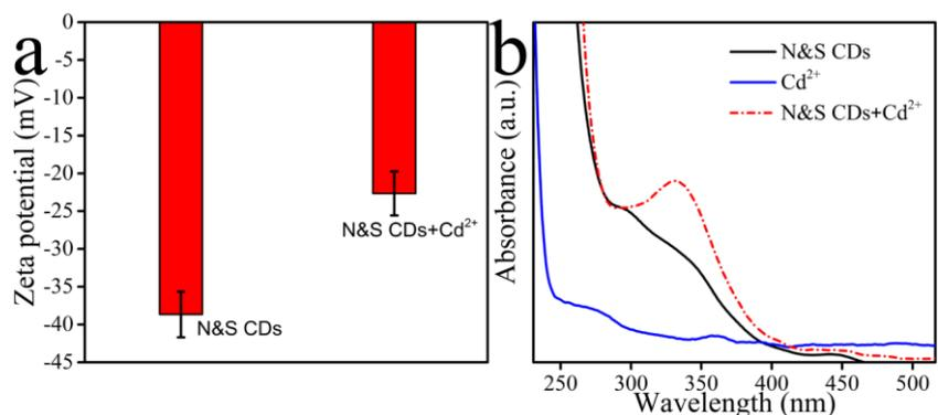
**Fig. S12** The zeta potential values of N&S CDs and N&S CDs+ $\text{Cd}^{2+}$  (a) and UV-vis absorption spectrum of N&S CDs with and without  $\text{Cd}^{2+}$  (b).
