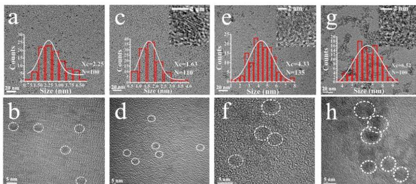
**Fig. S3** Optimized TEM images of synthesized N/S co-doping CDs under the reaction time of 2 h (a) and 4 h (c), with the amount 2-MT of 0.25 mM (e) and 1.00 mM (g), inserts are the corresponding particle size distribution. (b), (d), (f), (h) are the corresponding TEM in the scale of 5 nm.
