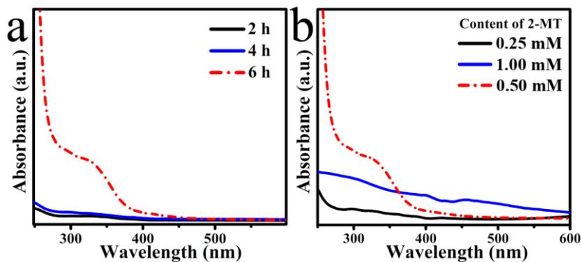
**Fig. S2** UV-vis absorption spectrogram of the CDs synthesized under different conditions.
