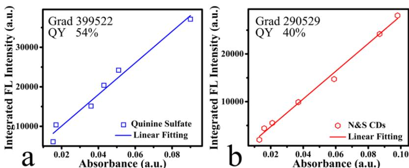
**Fig. S4** Plots of integrated PL intensity of quinine sulfate (a) and N/S CDs as a function of optical absorbance at 340 nm (b)
