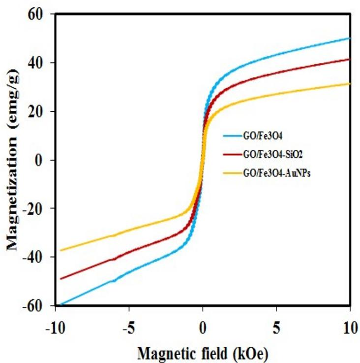
Fig. S1 VSM curves of GO/Fe<sub>3</sub>O<sub>4</sub>, GO/Fe<sub>3</sub>O<sub>4</sub>-SiO<sub>2</sub> and GO/Fe<sub>3</sub>O<sub>4</sub>-AuNPs
