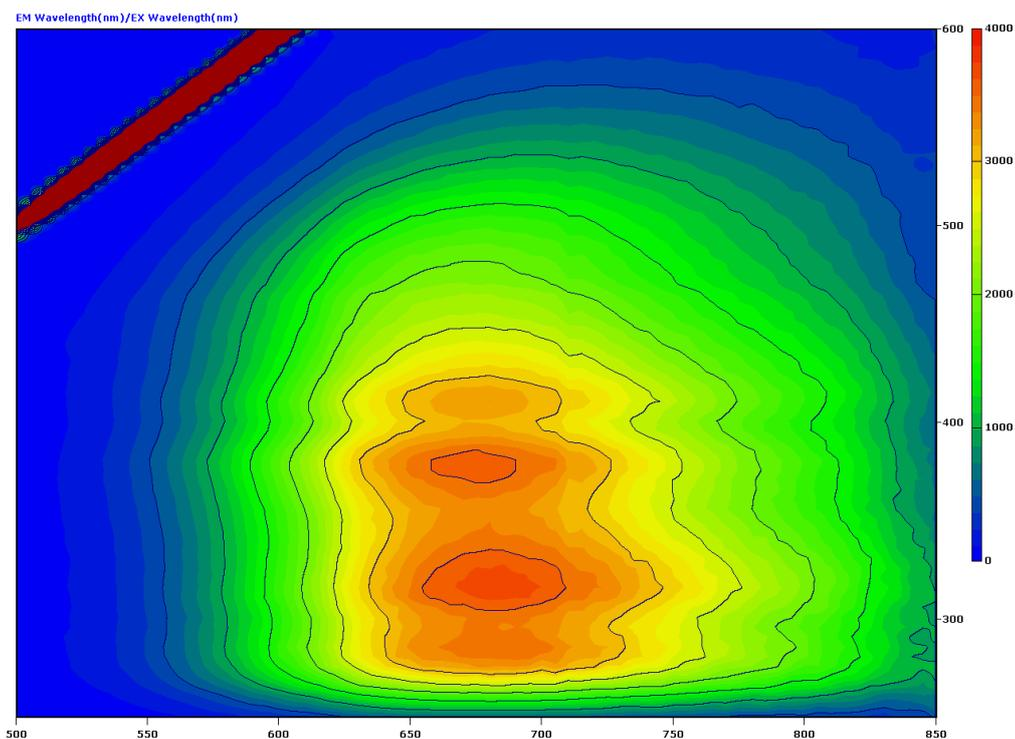
**Figure S2.** 2D fluorescence contour plot for the HSA-AgNCs complexes. (X-axis is emission and Y-axis is excitation).
