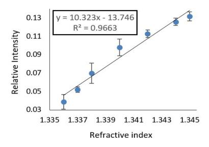
Fig.S3: The response of the sensor to different refractive index solutions
