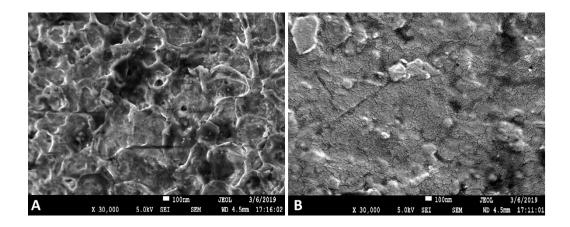
Fig. S1 FESEM images of A) Aptamer functionalized probe and B) Control gold probe
