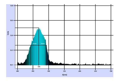
Fig.S2. Output wavelength evaluated using the image spectrum analyser
