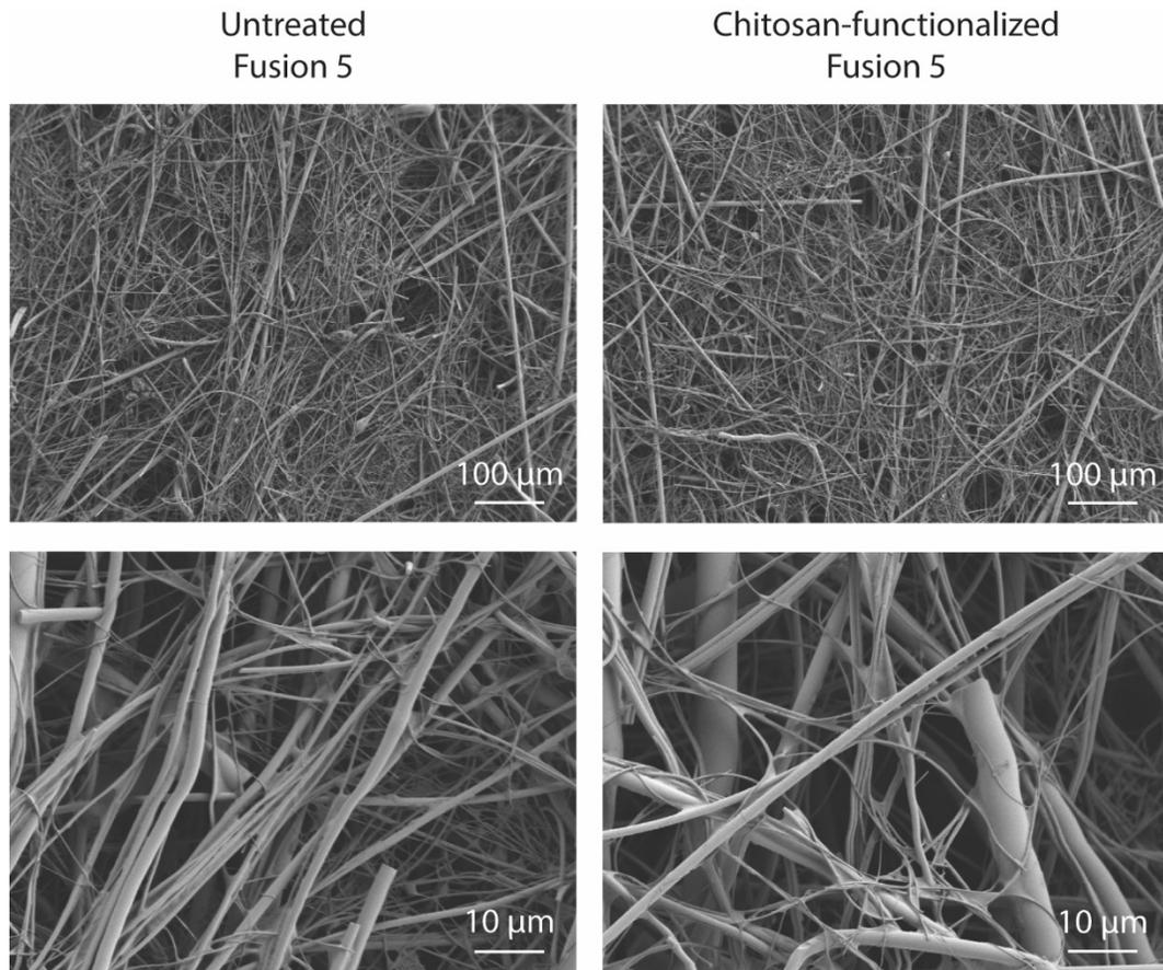
Samples of chitosan-functionalized and native Fusion 5 membranes were sputtered with gold (Cressington 108) and imaged via SEM (Zeiss Supra 40VP). No notable differences in morphology were observed between the treated and untreated conditions.
