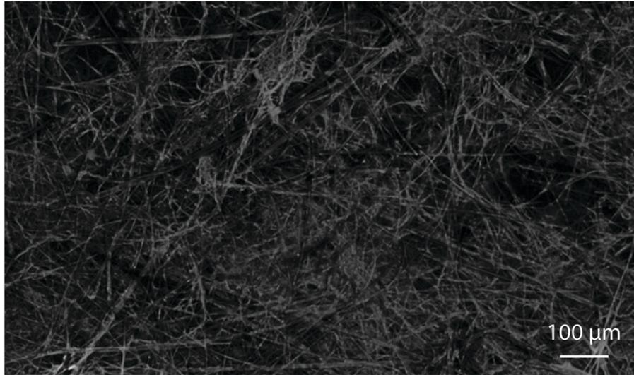
Fusion 5 membrane functionalized with FITC-tagged chitosan (see figure S2 for protocol) was soaked with Tris EDTA buffer pH 8.5 and imaged with a confocal microscope (Olympus FV3000) with excitation at 488 nm. 25 ROI were stitched together using ImageJ and the 3D viewer tool was used to assemble a 60 micron thick rendering of the membrane. The morphology of the fluorescently tagged chitosan is highly similar to the fibrous structure of the Fusion 5 substrate (figure S3).
