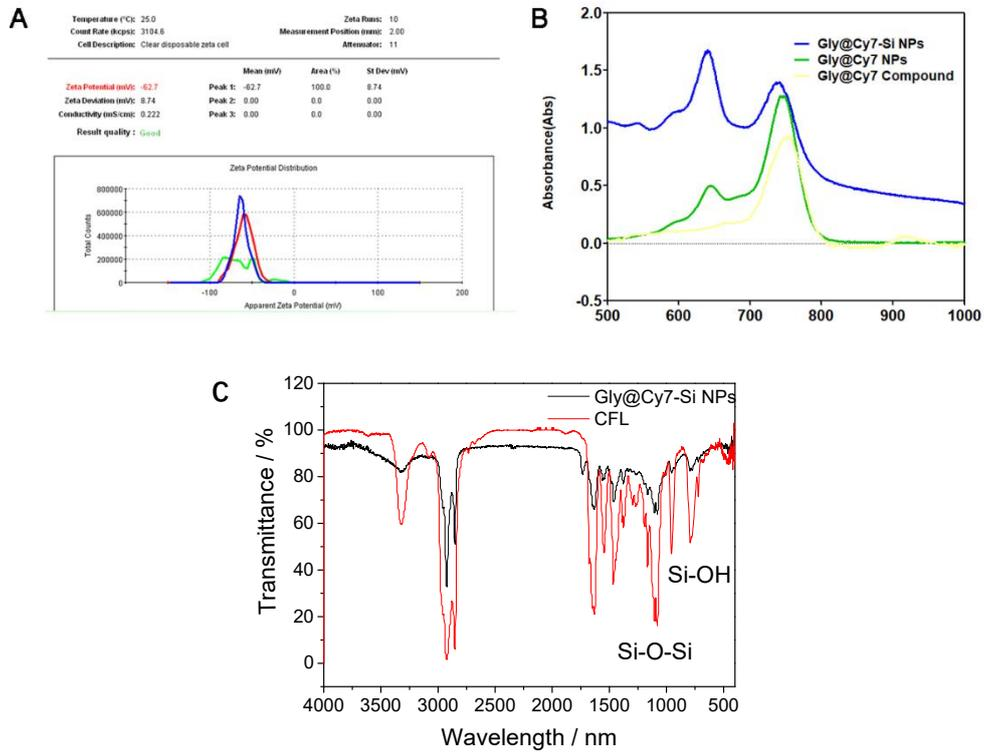
Figure S4: (A) Zeta-Potential of Gly@Cy7-Si NPs (B) UV-VIS spectra of Gly@Cy7 NPs, Gly@Cy7-Si NPs and Gly@Cy7 compound. (C) Fourier infrared spectroscopy of Gly@Cy7-Si NPs and CFL.
