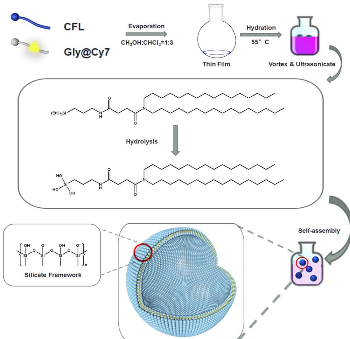
Figure S3: Schematic diagram of the synthesis of Gly@Cy7-Si nanoparticles.
