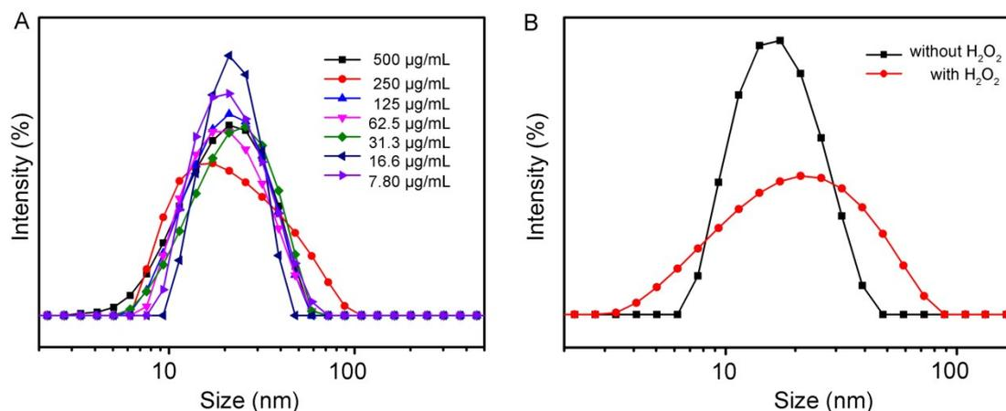
**Fig. S7.** The hydrodynamic radius of the mPEG-*b*-P(PA-*alt*-GPBAe) micelles (PAPBN) at the concentrations of 7.8–500  $\mu\text{g mL}^{-1}$  (A) and PAPBN before and after treatment with 200 mM  $\text{H}_2\text{O}_2$  for 24 h (B).
