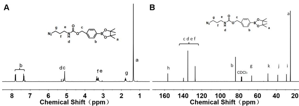
**Fig. S3.**  $^1\text{H}$  NMR (A) and  $^{13}\text{C}$  NMR (B) spectra of  $\text{N}_3\text{-PBAe}$  in  $\text{CDCl}_3$
