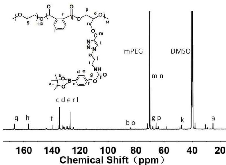
**Fig. S6.**  $^{13}\text{C}$  NMR spectrum of mPEG-*b*-P(PA-*alt*-GPBAe) in DMSO-*d*<sub>6</sub>.
