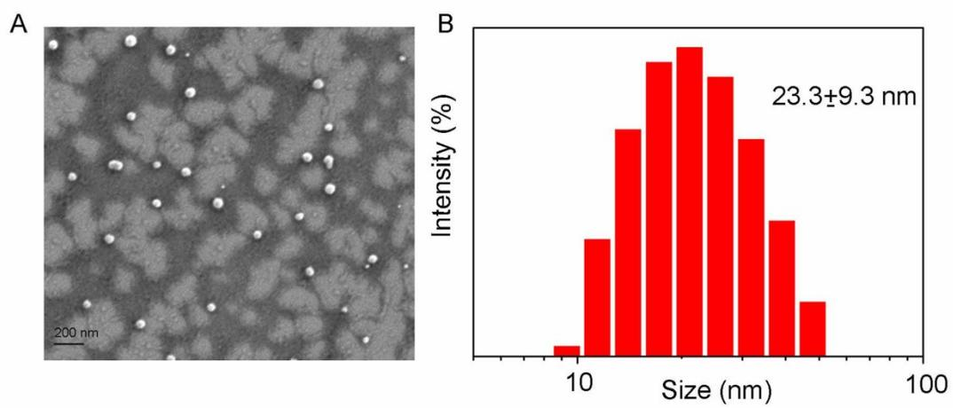
**Fig. S9.** The SEM image (A) and hydrodynamic radius (B) of PAPBN/DOX.
