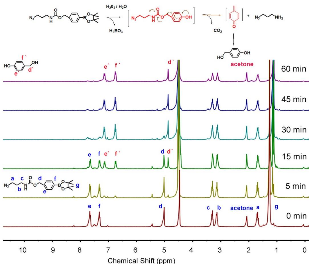
**Fig. S8.** Time-dependent  $^1\text{H}$  NMR spectra of  $\text{N}_3$ -PBAe oxidized by  $\text{H}_2\text{O}_2$  in acetone/ $\text{D}_2\text{O}$  ( $V/V=3:2$ ) with the  $\text{H}_2\text{O}_2/ \text{N}_3$ -PBAe molar ratio of 1:1 at room temperature.
