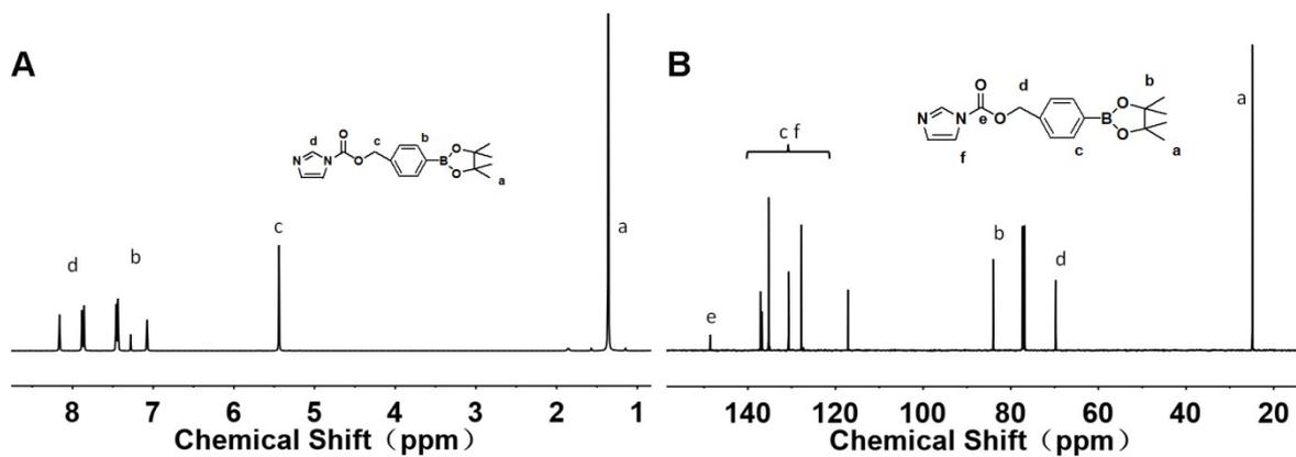
**Fig. S2.**  $^1\text{H}$  NMR (A) and  $^{13}\text{C}$  NMR (B) spectra of HPBAe-CDI in  $\text{CDCl}_3$ .
