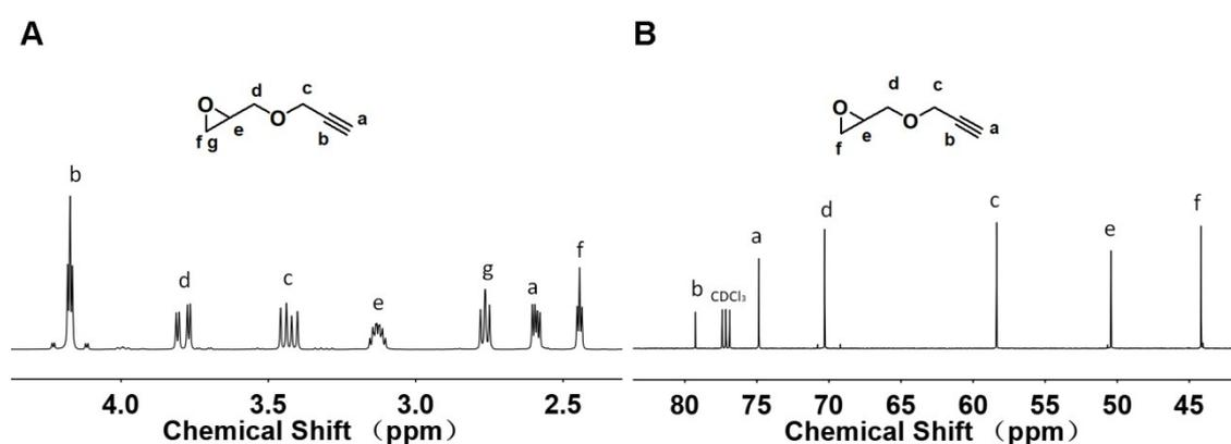
**Fig. S1.**  $^1\text{H}$  NMR (A) and  $^{13}\text{C}$  NMR (B) spectra of glycidyl propargyl ether (GPE) monomer in  $\text{CDCl}_3$ .
