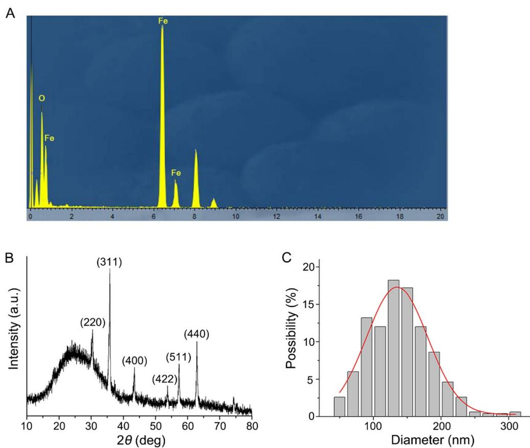
**Supplementary Figure 1.** Characterization of MIONs. (A, B) Energy-dispersive X-ray spectroscopy (A) and X-ray diffraction (B) confirm the nature of the clusters. (C) Size distributions of the samples.
