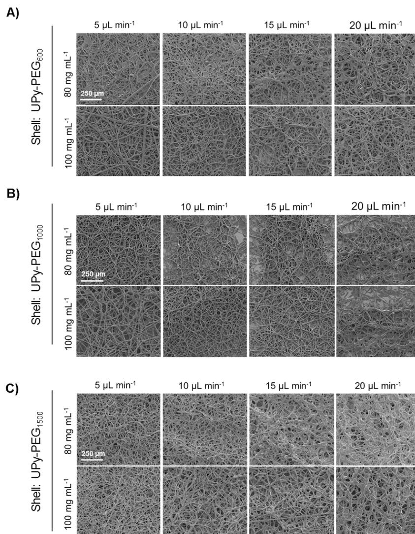
**Figure S2. Morphology of fibers fabricated by coaxial electrospinning.** SEM micrographs of core-shell fibers fabricated with a UPy-PC core solution with constant flow and concentration, and a shell UPy-PEG solution containing UPy-PEG<sub>600</sub> (A), UPy-PEG<sub>1000</sub> (B) or UPy-PEG<sub>1500</sub> (C). The flow rate and concentration of the shell solution were varied between 5 and 20  $\mu\text{L min}^{-1}$  and 80 and 100 mg mL<sup>-1</sup>. Scale bars represent 250  $\mu\text{m}$ .
