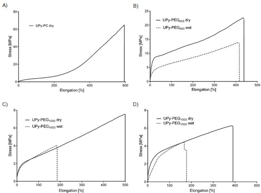
**Figure S1. Bulk tensile properties of polymers used in this study.** Representative tensile curves of polymers used in this study. A) UPy-PC; B) UPy-PEG<sub>600</sub> in dry (solid line) and wet (dashed line) conditions; C) UPy-PEG<sub>1000</sub> in dry (solid line) and wet (dashed line) conditions; D) UPy-PEG<sub>1500</sub> in dry (solid line) and wet (dashed line) conditions.
