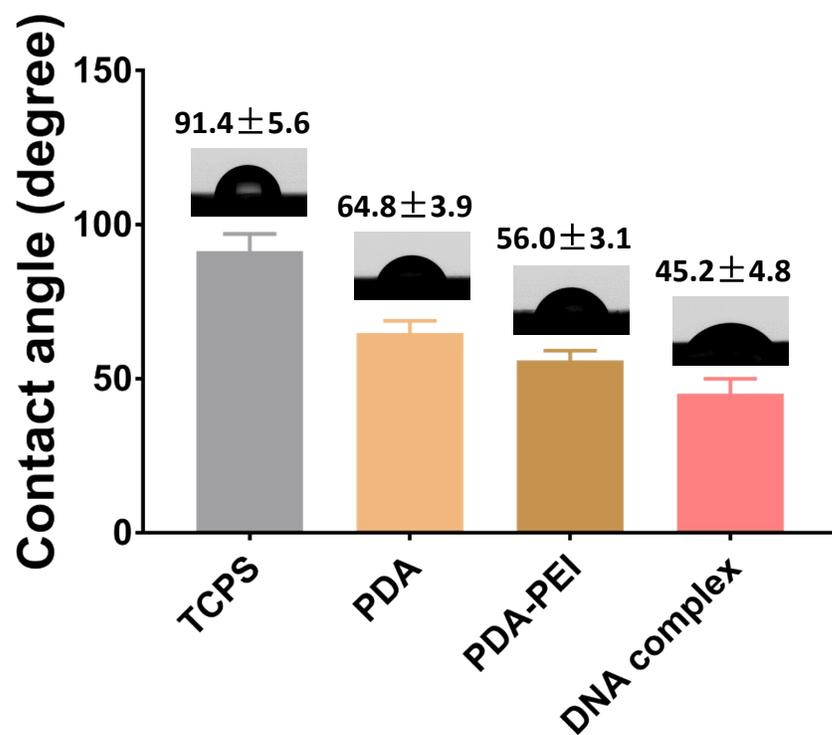
**Figure S1.** Water contact angles and digital photographs of water drops on TCPS, PDA, PDA-PEI, and pDNA-immobilized PDA-PEI surfaces. Experiments were repeated five times independently.
