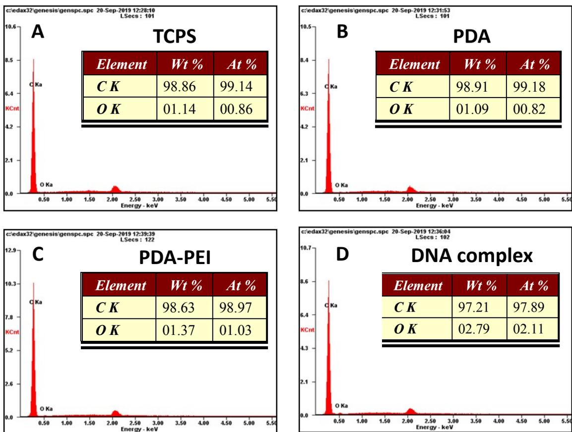
**Figure S2.** The elemental compositions of TCPS (A), PDA (B), PDA-PEI (C), and pDNA-immobilized PDA-PEI (D) surfaces examined by EDX.
