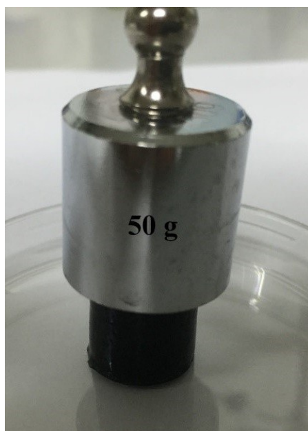
Figure S1. PEDOT 5 Alg 5 hydrogel is capable of bearing the 50 g of weight.
