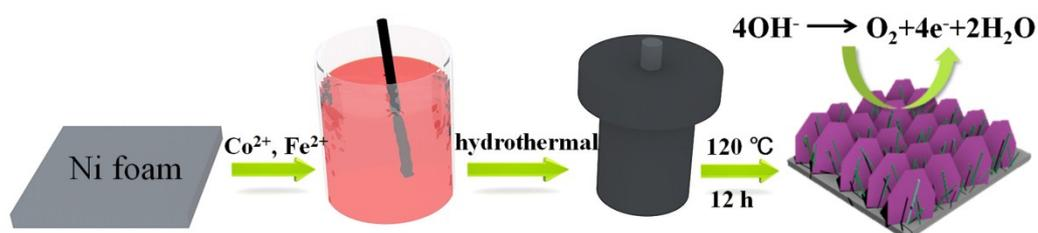
**Scheme S1.** Schematic representation of the fabrication procedure for  $\text{Co}_4\text{Fe}_2$ -LDHs/ $\text{Co}(\text{OH})_2$ -NWs with wire-in-plate structure via a simple one-step hydrothermal method
