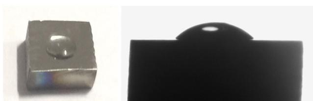
Fig. S6 Optical image of TC4 alloy and the WCA result
