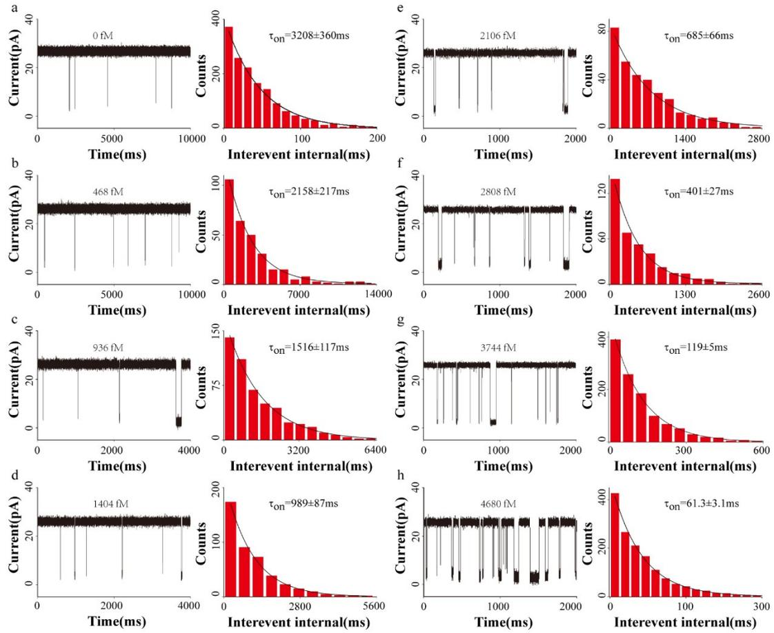
**Fig. S6** Representative single-channel current traces (left) and histogram of interevent interval ( $\tau_{\text{on}}$ , right) of  $\text{IP}_6$  through a  $\alpha\text{-HL(M113R)}_7$  nanopore recorded with different biotin-TRF concentration. The experiments were performed at +30 mV in 10 mM Tris solutions containing 1 M KCl (pH 7.4). The concentration of biotin-TRF increased from (a) 0 fM, (b) 468 fM, (c) 936 fM, (d) 1404 fM, (e) 2106 fM, (f) 2808 fM, (g) 3744 fM, (h) 4680 fM.
