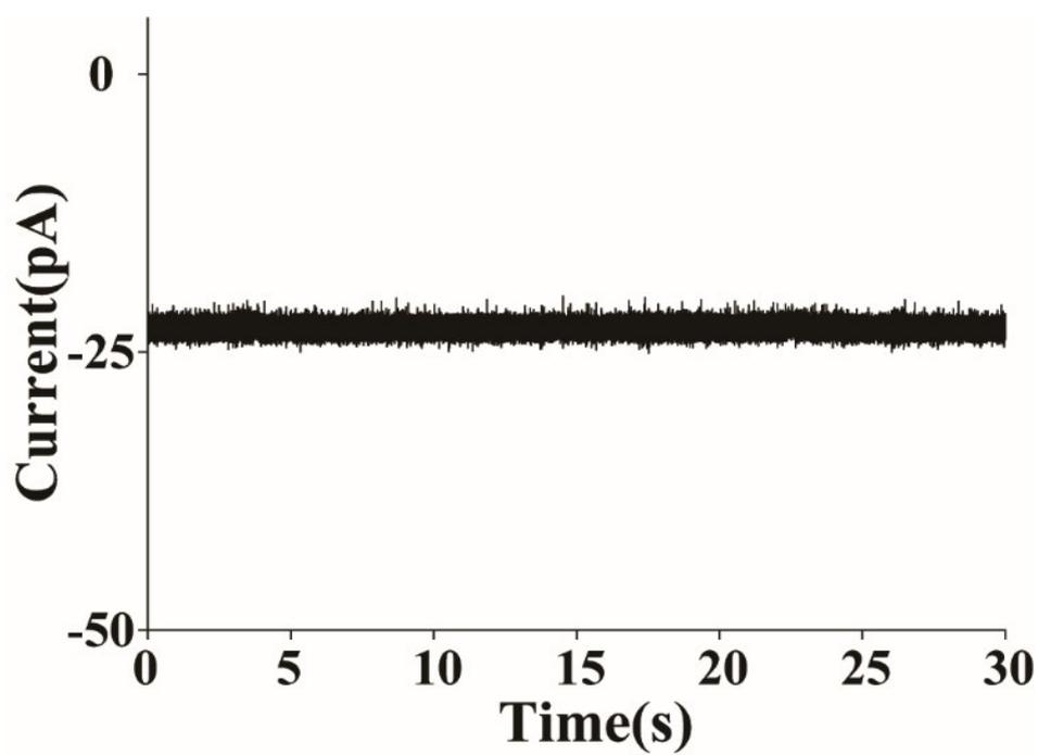
**Fig. S2** Representative current trace recorded when IP<sub>6</sub> capsulated SUVs were added in the trans-side of the chamber, and bias potential was -30 mV. No transfer event was detected. The trace was recorded with 1.25 ug/mL SUVs, 1M KCl, and 10mM Tris (pH=7.4).
