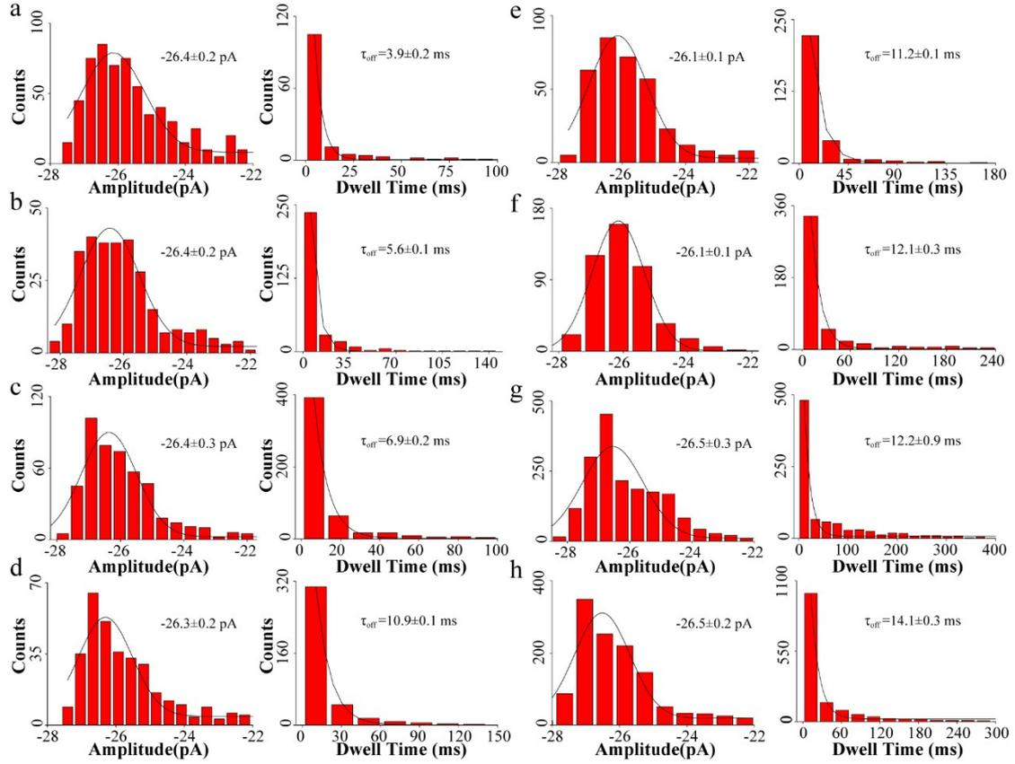
**Fig. S8** Representative histogram of current (left) and dwell time ( $\tau_{\text{off}}$ , right) of IP<sub>6</sub> through a  $\alpha$ -HL(M113R)<sub>7</sub> nanopore recorded with different biotin-TRF concentration. The experiments were performed at +30 mV in 10 mM Tris solutions containing 1 M KCl (pH 7.4). The concentration of biotin-TRF increased from (a) 0 fM, (b) 468 fM, (c) 936 fM, (d) 1404 fM, (e) 2106 fM, (f) 2808 fM, (g) 3744 fM, (h) 4680 fM.
