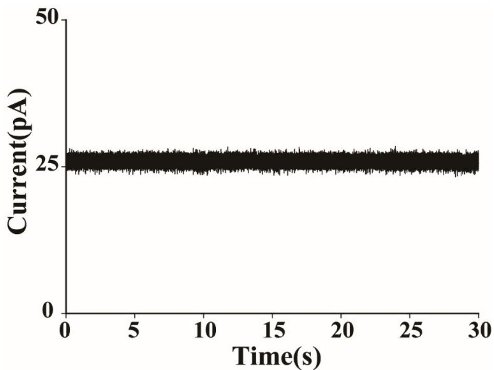
**Fig. S3** Representative current trace recorded when 60  $\mu\text{L}$  aqueous solution out of dialysis bag after the last dialysis was added in cis side chamber. The bias potential was +30 mV. No transfer event was detected. The trace was recorded with 1M KCl, and 10mM Tris (pH=7.4).
