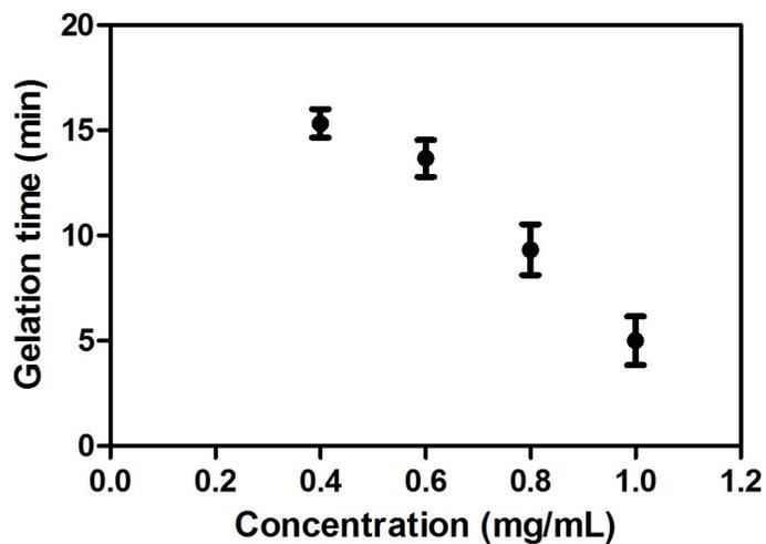
**Fig. S9.** Gelation time of compound **3** by ESAI at different concentration from 4 °C to 37 °C
