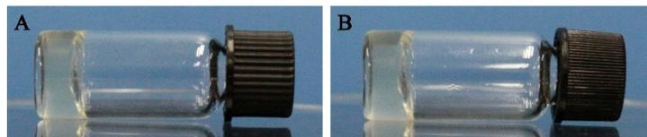
**Fig. S10.** Optical images of thermogel of **2** after being put back to 4 °C for A) 15 minutes and B) 12 hours.
