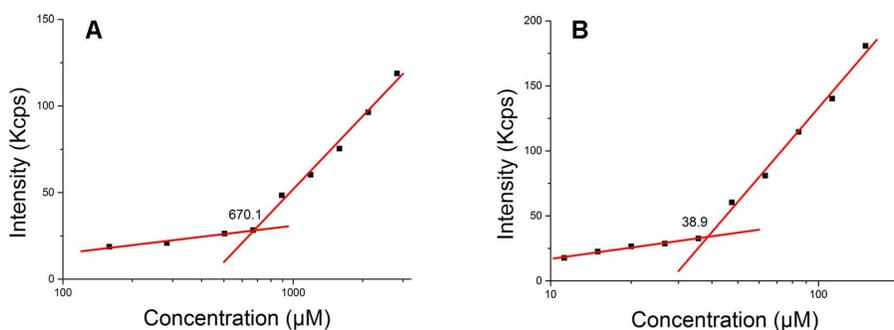
**Fig. S7.** Critical aggregation concentration (CAC) value of compound **3** at A) 4 °C and B) 37 °C
