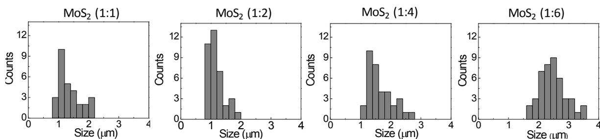
**Figure S1:** The size-distribution presented by histograms shows the cumulative counts of three pictures for each sample from 1:1 to 1:6. The representative images are presented in figure 1c. The results indicate the avg. size to be about 1.5-3  $\mu\text{m}$  for each nanoflower with slight rise due to increase in sulfur precursor from  $\text{MoS}_2$  (1:1) through  $\text{MoS}_2$  (1:6).
