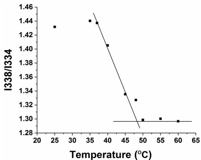
**Fig. S1** Characterization of LCST of PNIPAM-based nanoparticles by pyrene fluorescence spectroscopy.
