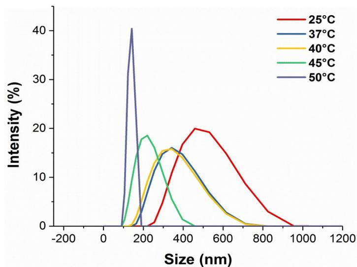
**Fig. S2** Characterization of particle size changes at different temperatures for PNIPAM-PTX.
