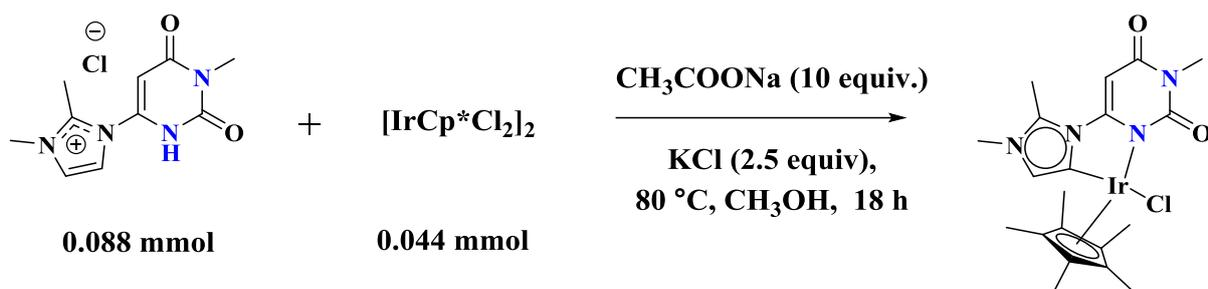
**Scheme S4.** Synthesis of Ir-U<sub>NMe</sub>
