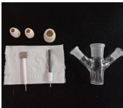
**Figure S1.** The experimental setup for electrolysis.
