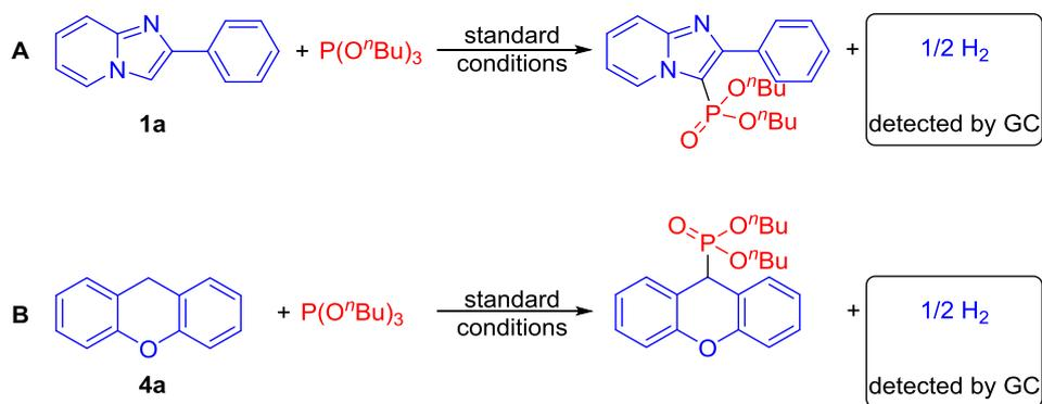
When reaction was finished, the gas mixture was analyzed by GC and H<sub>2</sub> could be detected.
