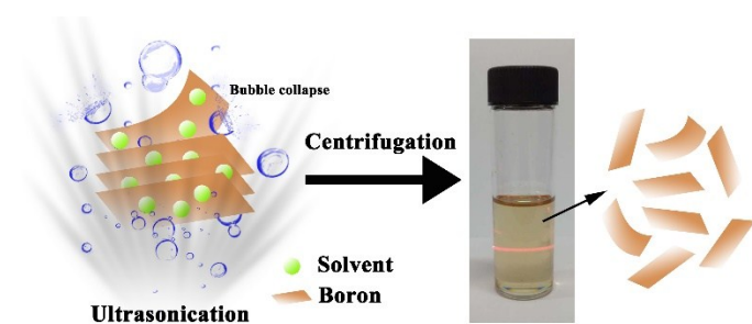
Fig. S1 Schematic illustration of ultrasonication-assisted liquid-phase exfoliation of boron. The photograph shows a Tyndall effect of the boron nanosheet dispersion, an indication of a colloidal stable nature.
