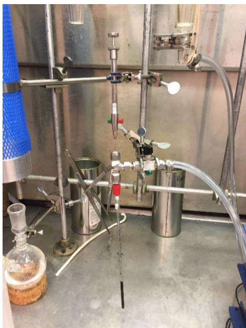
**Figure S11.** Apparatus for J.Young tube headspace sampling with gas tight syringe.
