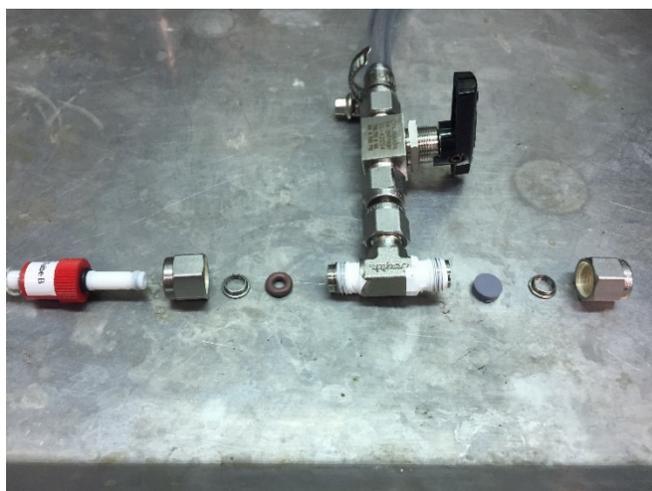
**Figure S10.** Disassembled apparatus for J.Young tube headspace sampling.
