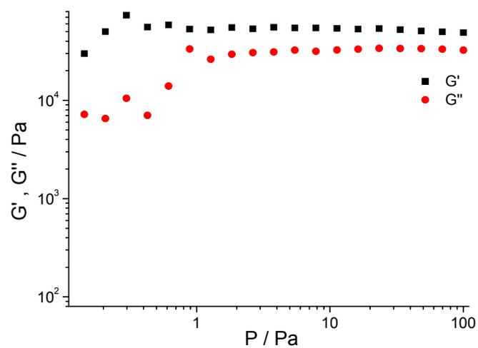
**Fig. S5** Plots of storage modulus ( $G'$ ) and loss modulus ( $G''$ ) against applied shear stress on the PVP/ $\text{CH}_2\text{Cl}_2$  gel. The measurement shear frequency was fixed at 1 Hz.
