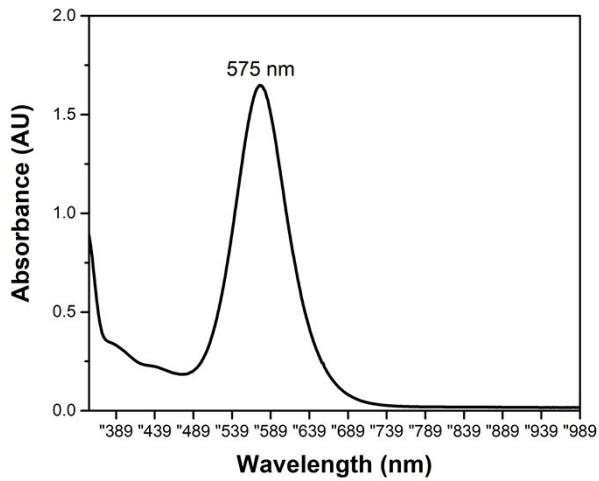
**Fig S2.** UV spectrum of compound **2** in n-hexane
