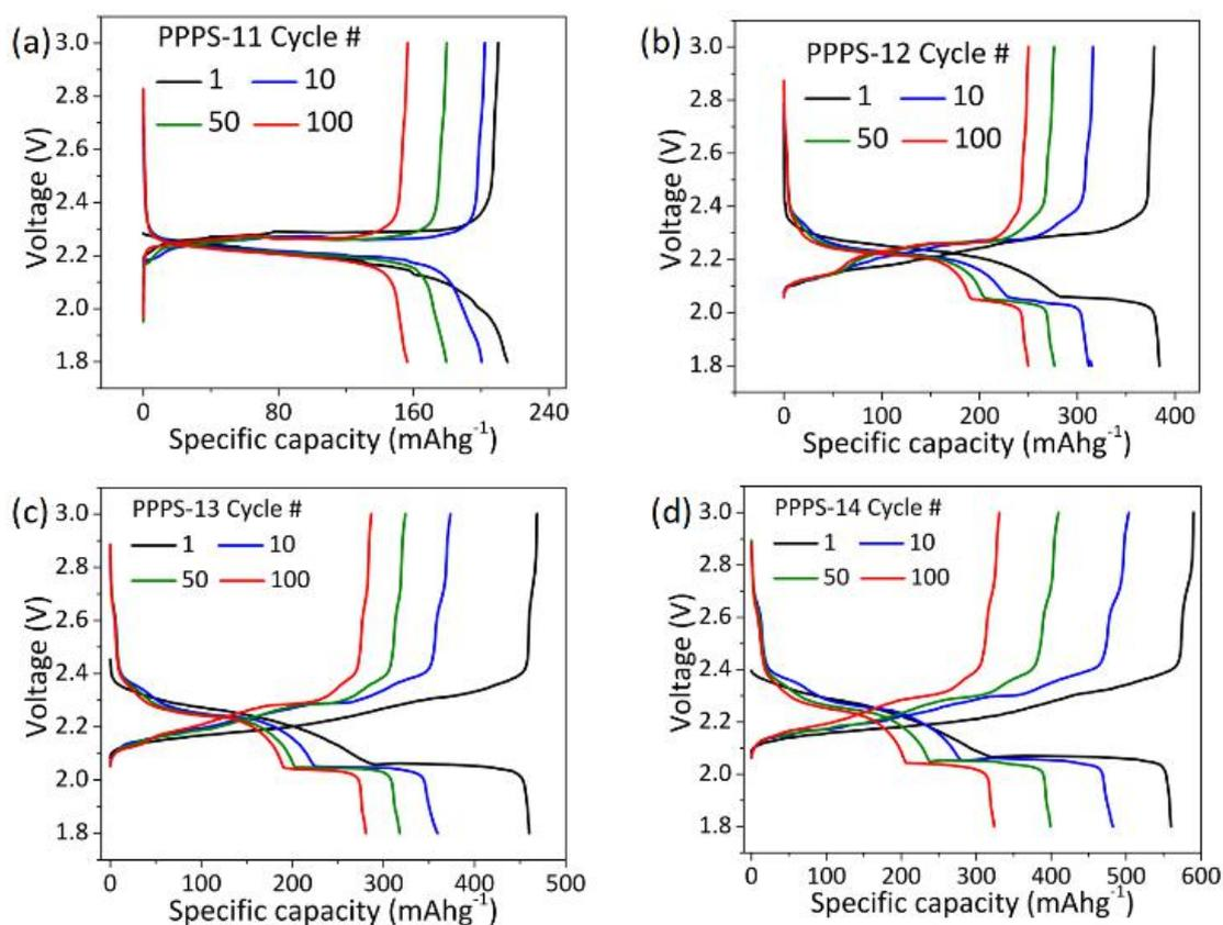
**Figure S5.** Discharge and recharge voltage profiles of cells with (a) PPS-11, (b) PPS-12, (c) PPS-13, and (d) PPS-14 cathodes at different cycles.
