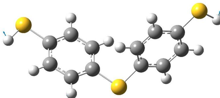
**Figure S2.** The optimized molecular structure and harmonic vibrational frequencies of 4,4'-thiobisbenzenethiol were calculated using density function theory (DFT) at M06-2X/6-31+G (d, p) level by Gaussian 09 software.<sup>1</sup> The nuclear displacements of the bending vibration of -SH group are shown in blue arrows. Carbon atoms are gray, hydrogens gray-white and sulfur yellow.
