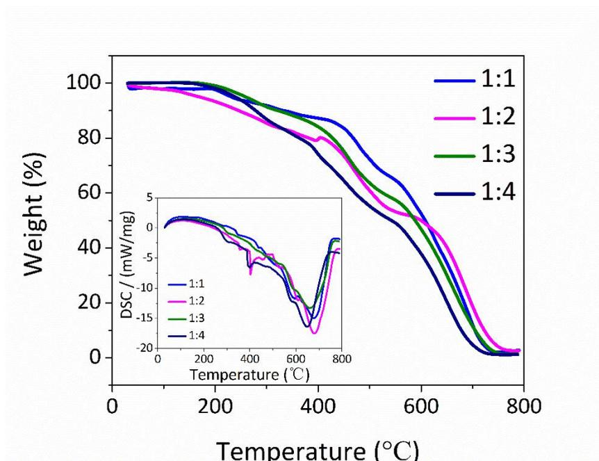
**Figure S3.** TGA and DSC plots of the cast polymers.
