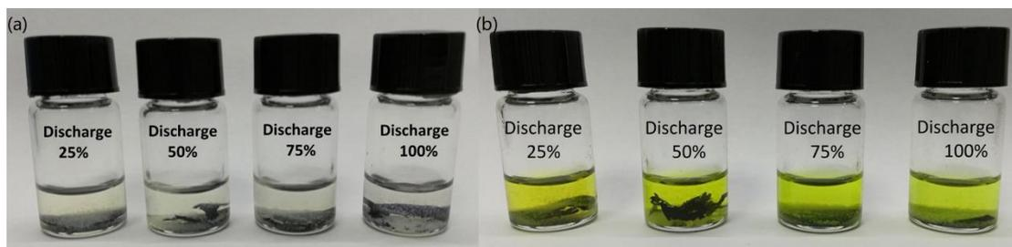
**Figure S4.** (a) PPPS-11 and (a) PPPS-13 electrodes in DME in the discharge state of 25%, 50%, 75%, and 100%.
