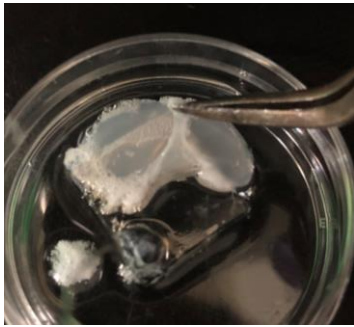
Fig. S3 Fibrin gel electrodeposited on a large electrode. Volume: 1 mL. Applied potential: 3 V. Applied time: 2 min. Incubation time: 13 min.
