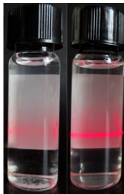
Fig. S6 Tyndall effect (left) before and (right) after exfoliation.
