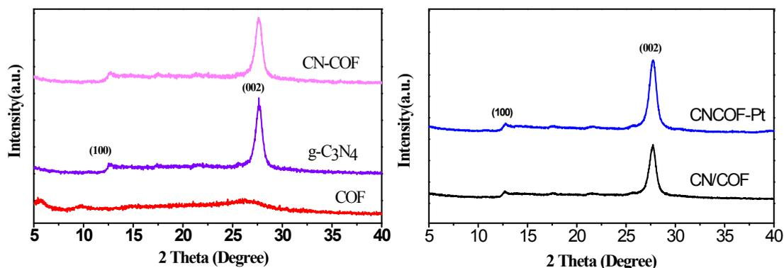
**Figure S4.** Powder X-ray diffraction pattern of (left) g-C<sub>3</sub>N<sub>4</sub>, COF, CN-COF, and (right) CN/COF and CNCOF-Pt.
