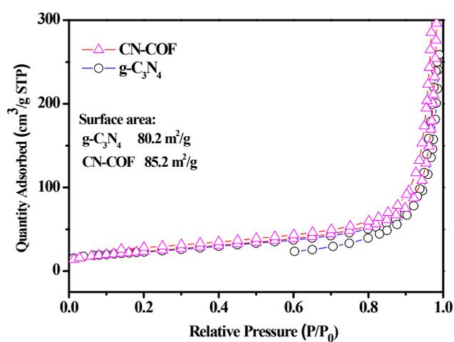
**Figure S6.**  $\text{N}_2$  adsorption-desorption isotherm of  $g\text{-C}_3\text{N}_4$  and CN-COF.
