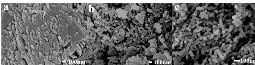
**Figure S11.** SEM images of g-C<sub>3</sub>N<sub>4</sub> (a), CN-COF (b), and COF (c).
