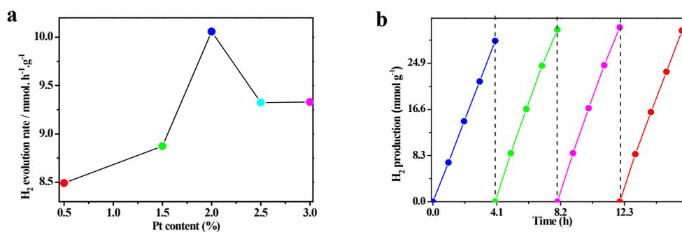
**Figure S9.** (a) H<sub>2</sub> production rate of CN-COF (3%)-Pt (x%). (b) Photocatalytic stability test of CN-COF.
