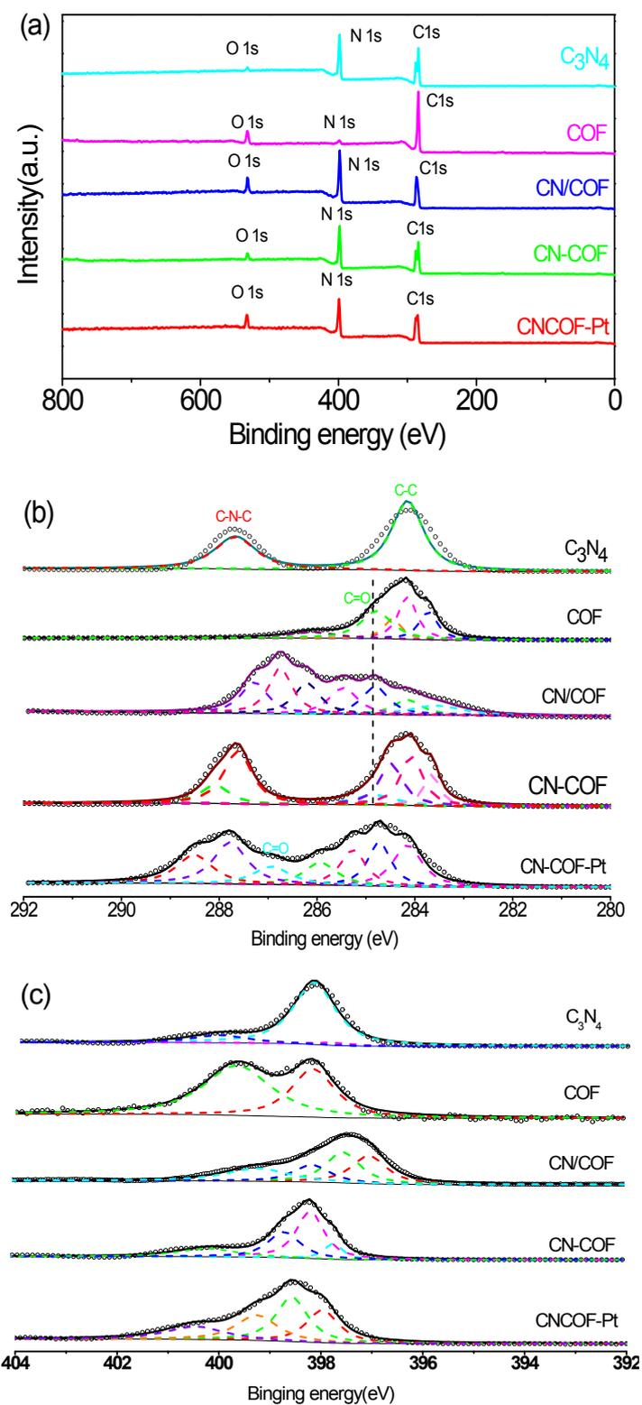
**Figure S2.** XPS spectra of the samples. (a) The survey scan, (b) High-resolution spectra of C 1s for samples, and (c) High-resolution spectra of C 1s for the samples.
