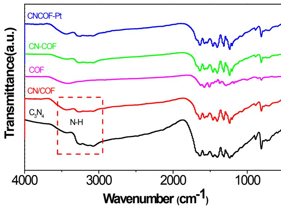
Figure S1. FT-IR spectra of g-C<sub>3</sub>N<sub>4</sub>, COF, CN/COF, CN-COF and CNCOF-Pt.
