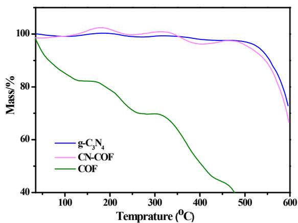
**Figure S5.** Thermal gravimetric analysis of  $g\text{-C}_3\text{N}_4$ , COF and CN-COF.
