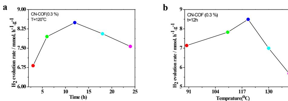
**Figure S10.** H<sub>2</sub> production rate of CN-COF prepared at different reaction time and temperature.
