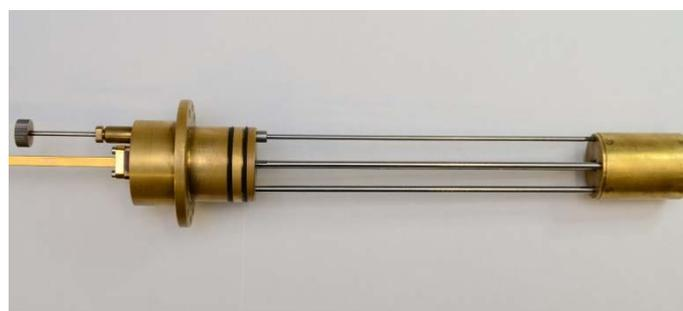
**Figure S 2:** Closed FPR, the flange on the top complies with our flow cryostat
