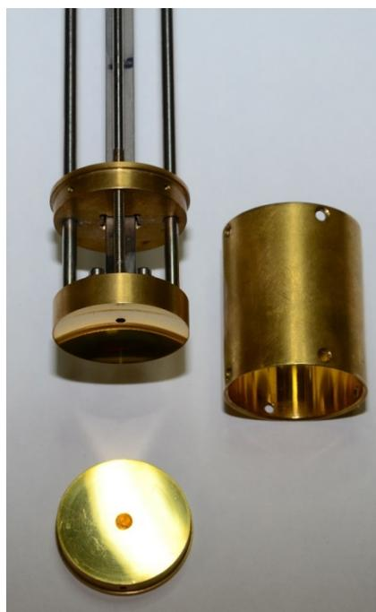
**Figure S 1:** Opened, manufactured FPR with a 5 mm diameter sample mounted.
