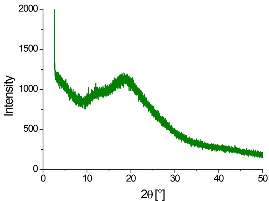
**Figure S3.** Powder X-ray diffraction (PXRD) pattern of **CX4-NC**.
