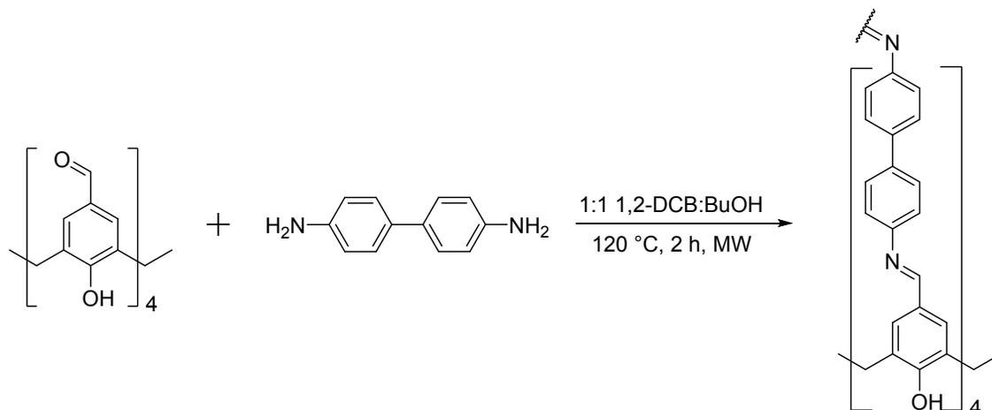
**CX4-NC synthesis.** 25.0 mg of CX4-CHO was dissolved in 2.5 mL of 1,2-dichlorobenzene and 2.5 mL of 1-butanol, and the mixture was added to 17.0 mg of benzidine in a 8-mL microwave reactor tube. 100 μL of 6M acetic acid was added as a catalyst. The reaction was performed in CEM Discover SP microwave reactor at 120 °C for 2 h with high stirring. The contents of the reaction vessel were centrifuged and repeatedly washed with ethanol. The solid was dried in a vacuum oven at 40 °C overnight.
