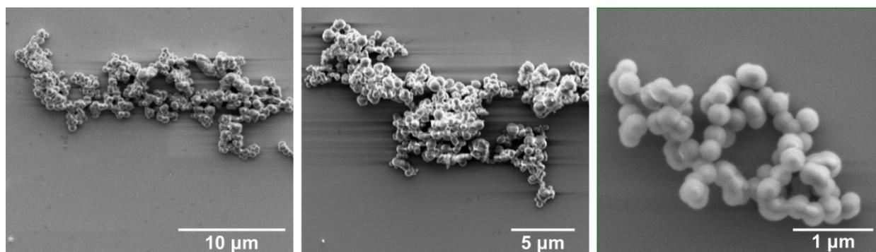
**Figure S5.** Evaluation of stability of **CX4-NC** in PBS. SEM images obtained after 48 h incubation in PBS at room temperature.
