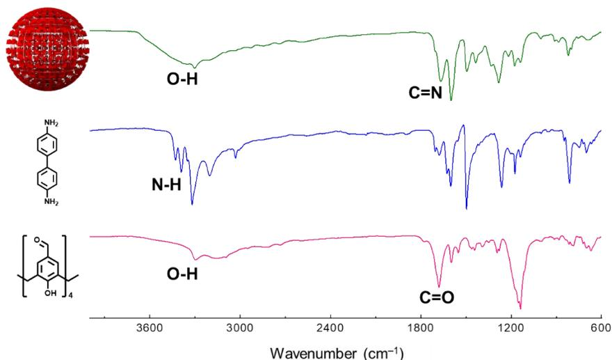
**Figure S1.** FTIR spectra of **CX4-NC** and corresponding monomers, CX4-CHO (1) and benzidine (2).
