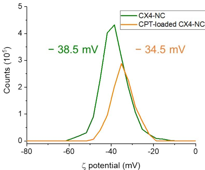
**Figure S10.** ζ potential for **CX4-NC** before and after CPT loading.
