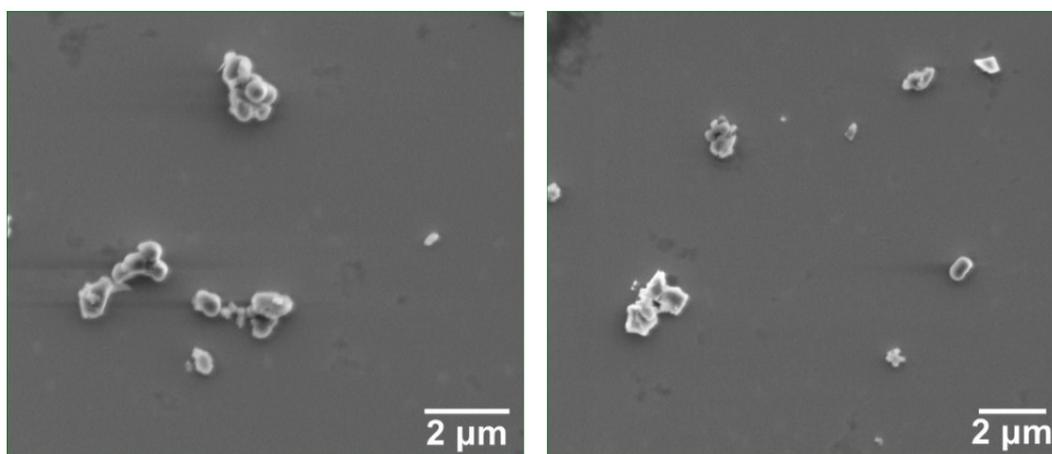
**Figure S12.** SEM images of **CX4-NC** after CPT release at acidic conditions.
