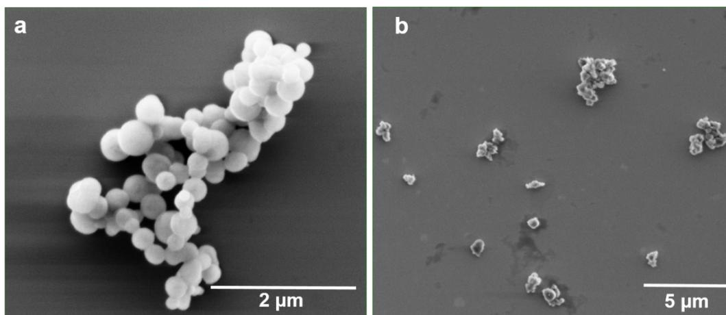
**Figure S13.** SEM images of **CX4-NC** at different stages of CPT release in presence of GSH. In early stages (a, t = 2 h), the morphology of capsules is preserved, but over time (b, t = 48 h) NCs disintegrate.
