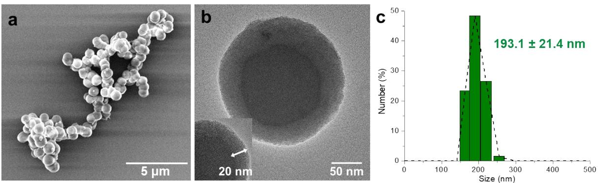
**Figure S2.** Characterization of as-synthesized **CX4-NC**. SEM micrograph (a), TEM micrograph (b) and size distribution measured by DLS (c). Inset shows the shell thickness of **CX4-NC**.
