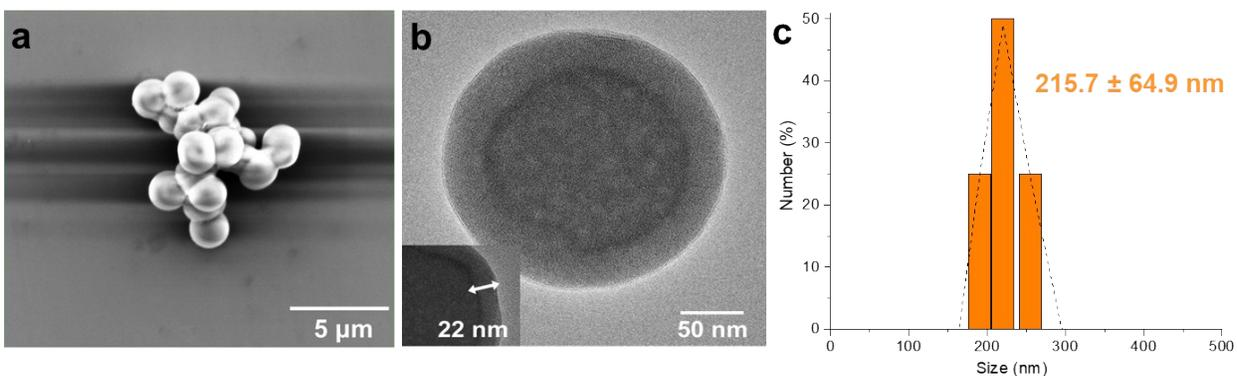
**Figure S8.** Characterization of **CX4-NC** after CPT loading. SEM micrograph (a), TEM micrograph (b) and size distribution measured by DLS (c) of post-synthetically CPT-loaded **CX4-NC**. Inset shows the shell thickness of **CPT-CX4-NC**.
