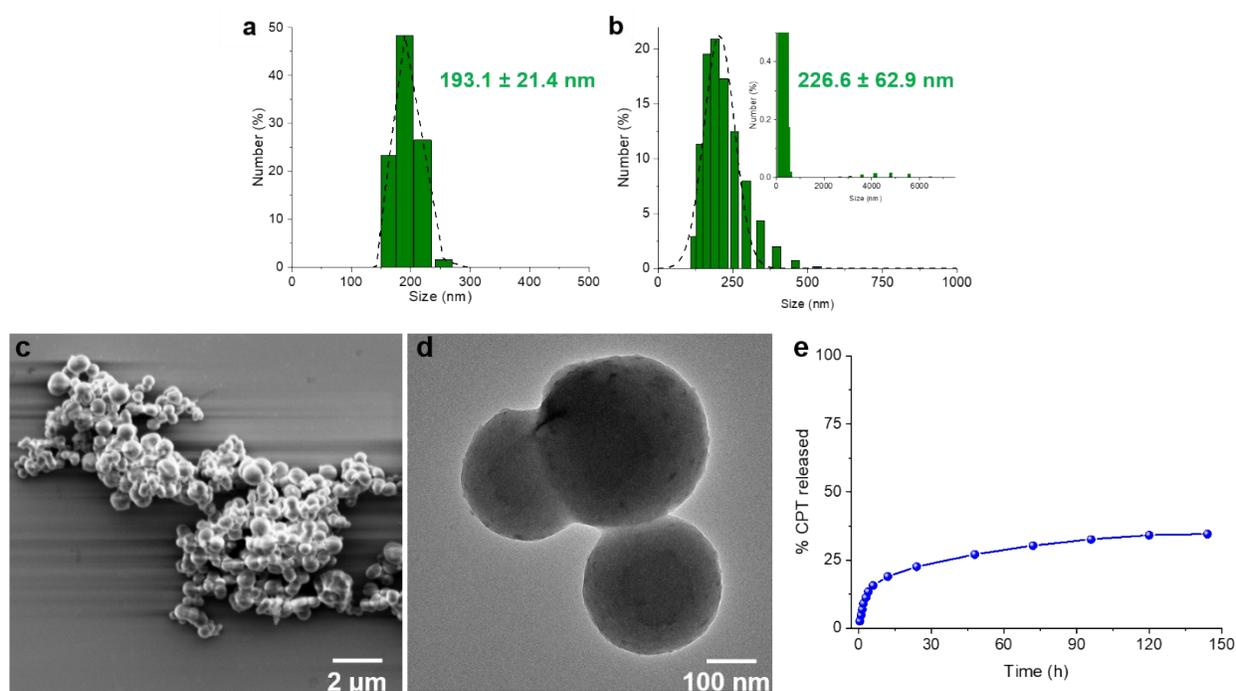
**Figure S6.** DLS measurements of as-synthesized **CX4-NC** dispersed in PBS (a) and following a 48h incubation in PBS (b). Evaluation of stability of **CPT-CX4-NC** at 37 °C in PBS. (c) SEM and (d) TEM images of **CX4-NC** obtained after 48 h incubation. (e) Drug release profile of **CPT-CX4-NC** incubated in PBS at 37 °C.
